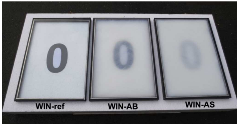
Figure 2.17: Aerogel glazing units from the work of Gao et al [52]. WIN-ref: no silica aerogel particles. WIN-AB: silica aerogel particles with sizes between 3 and 5 mm. WIN-AS: silica aerogel particles with sizes below 0.5 mm.
