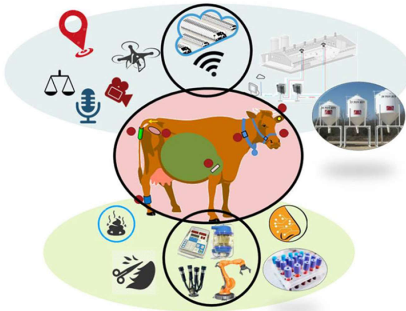
Figure 1. 11 Extracted from (Knight, 2020a). Overview of sensor technologies associated with dairy animals (can be extended to suckling breeds). The red zone and individual red dots show 'At Cow' sensors, the blue zone shows 'Near Cow' sensors and the green zone shows 'From Cow' sensors.
