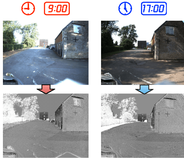
Figure 2.11: Improving image similarity at two different times of the day [Maddern 2014]. The RGB color model is converted to the illumination invariant color space using Equation (2.4).
