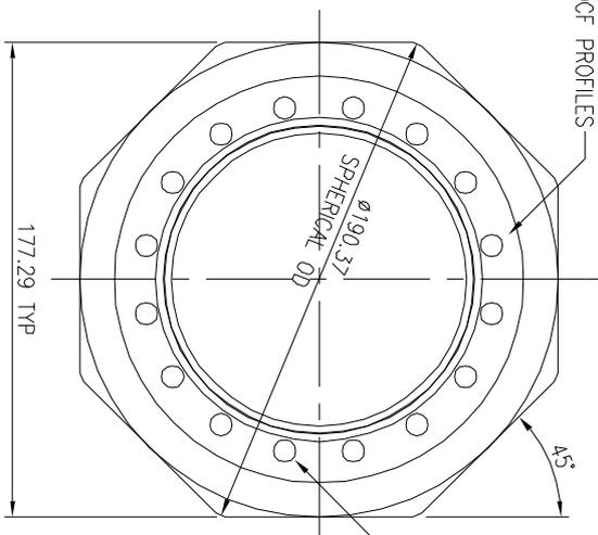
16 HOLES Ø8.4 THRU' EQUISPACED ON A 130.2±0.1 PCD AS SHOWN. CSK BOTH SIDES TO REMOVE BURRS
