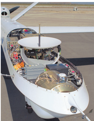
Figure 2.8: Close-up on the dish used for satellite communication in a NOAA-NASA MALE Reaper drone. The dish is mounted on a steerable mount, pointing upwards, allowing to aim specific satellites.
