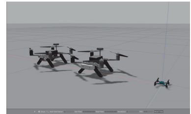
Figure 3.1: Two Intel Aero UAV and one Crazyflie drones simulated in Gazebo. Courtesy of Vincent Le Doze.
