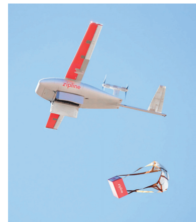
Figure 2.5: A ZipLine fixed-wing drone used to deliver medical materials and blood, using a parachuted package.
