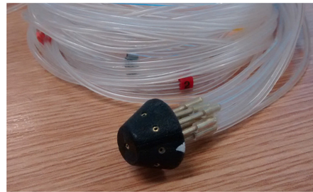
(B) Assembly of barnacle model prior to installation on blade model surface.
