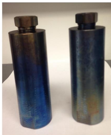
Figure 2.5: Two Ti alloy grade 2 reactors used for the supercritical synthesis at the University of Texas at Austin.
