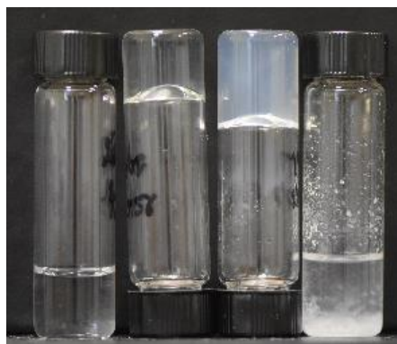
Figure 2.7. 75C12 aqueous solutions. From left to right: clear solution, clear gel, turbid gel and phase separation.
