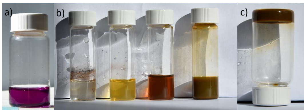
Figure 2.10. a) 1 g/L C_{60} solution in toluene. b) C_{60} aqueous colloidal suspensions. From left to right, concentrations are 1 mg/L, 25 mg/L, 0.26 g/L, 1.6 g/L. c) Hydrogel with C_{pol}=50 g/L and 0.8 g/L C_{60} .
