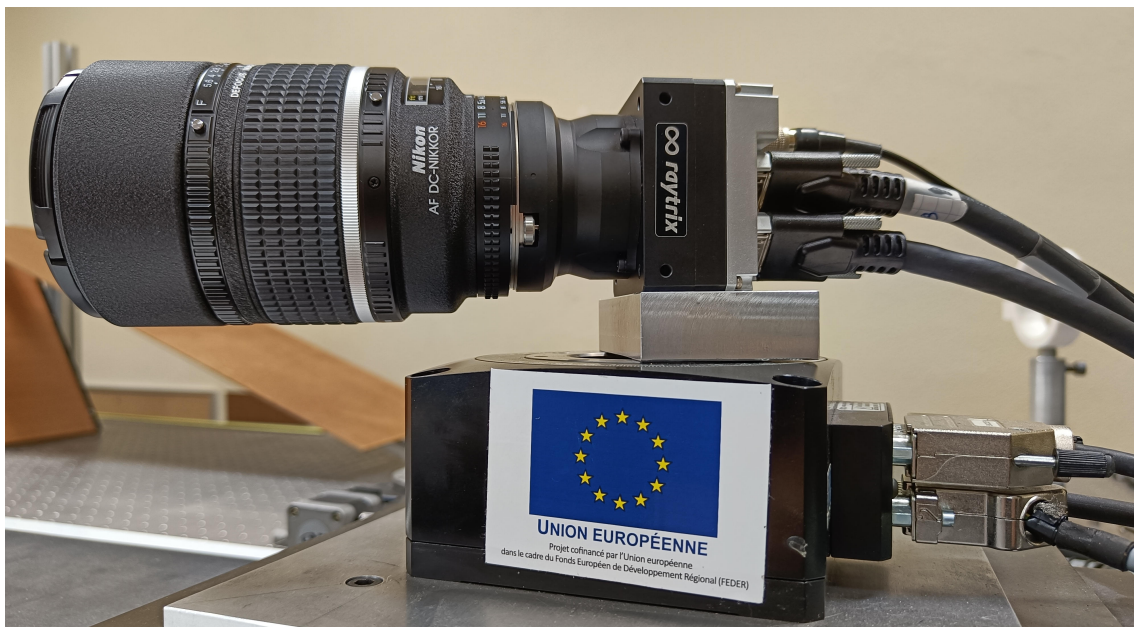
Figure B.7: Our Raytrix R12 plenoptic camera with the mounted lens of 135 mm focal length used in dataset R12-D.
