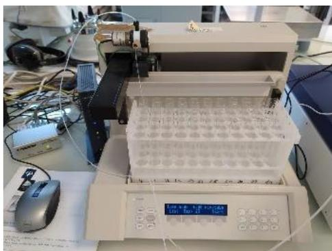
**Figure 2-5.** The FC-203B fraction collector.
