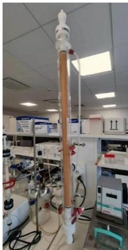
**Figure 2-3.** The YMC-ECO 25 column with UMA 150 resin inside.
