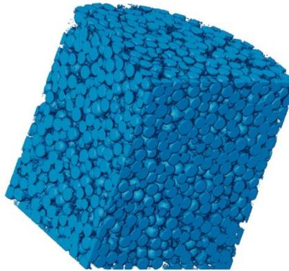
Figure 3-3. Part of resin bed (1/4 of a cylinder sample with 2mm of height) scanned by tomography.
