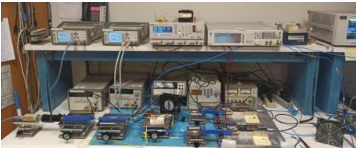
Figure 5.5: Photo of testbench of dual-input Doherty PA
