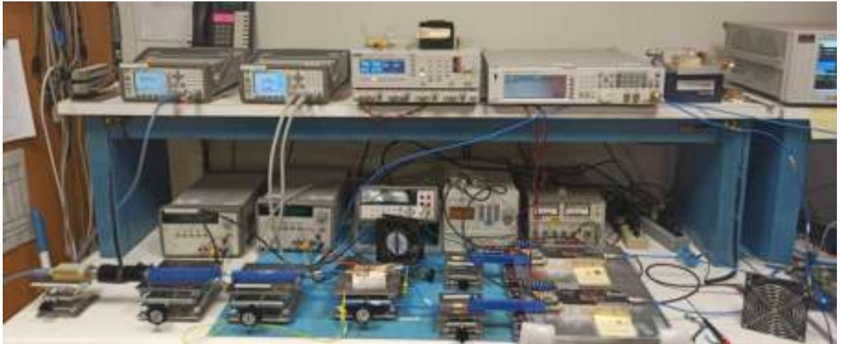
Figure 5.5: Photo of testbench of dual-input Doherty PA
