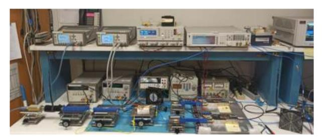
Figure 5.5: Photo of testbench of dual-input Doherty PA
