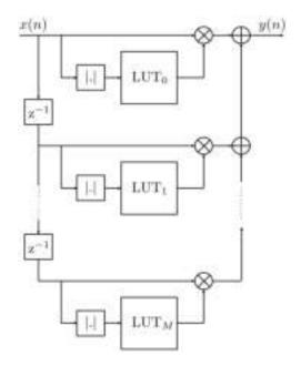
Figure 4.9: Architecture of LUT method to calculate polynomial
