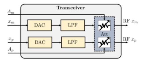
Figure 5.9: Block diagram of transceiver
