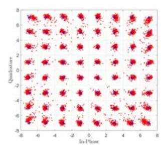
Figure 1.12: Constellation of input-output IQ data with EVM=10%
