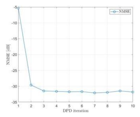
Figure 5.22: Evolution of NMSE according to DPD iterations
