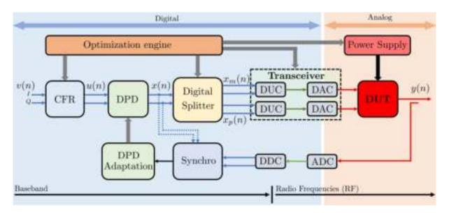
Figure 5.6: Block diagram of the proposed architecture
