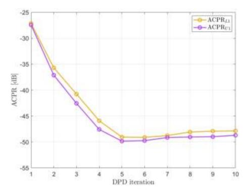
Figure 5.25: ACPR<sub>L1</sub> and ACPR<sub>U1</sub> versus DPD iterations
