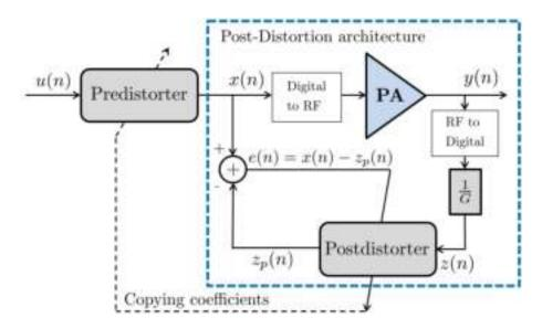
Figure 2.3: ILA and Post-Distortion architecture
