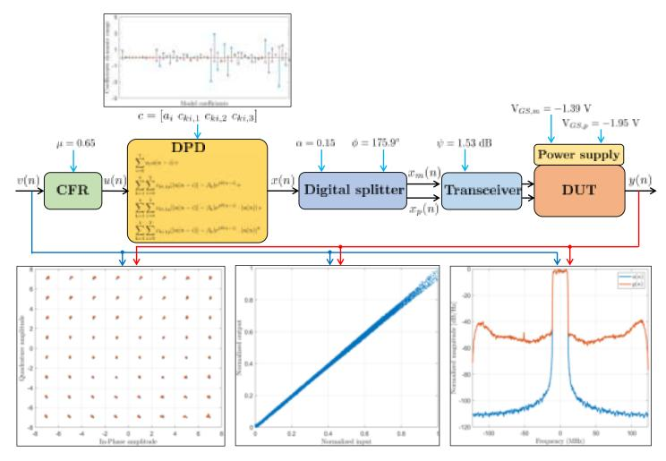
Figure 5.33: Final optimal configuration with DPD
