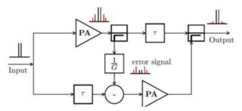
Figure 1.14: Principle of Feedforward
