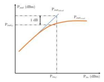
Figure 1.5: 1-dB compression point on AM-AM characteristic
