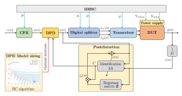
Figure 5.13: Integration of DPD using ILA to the entire system
