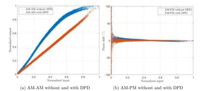
Figure 5.27: Characteristics of dual-input Doherty PA without and with DPD
