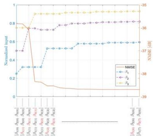
Figure 3.15: Evolution of thresholds and NMSE versus iterations
