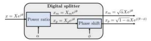
Figure 5.8: Block diagram of digital splitter
