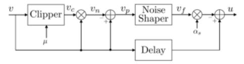
Figure 5.7: Block diagram of peak cancellation technique
