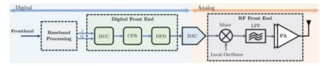
Figure 1.1: Block diagram of RF wireless transmitter
