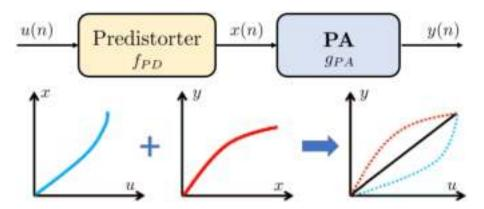
Figure 2.1: Principle of digital predistortion
