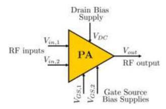
Figure 8: Block diagram of dual-input PA
