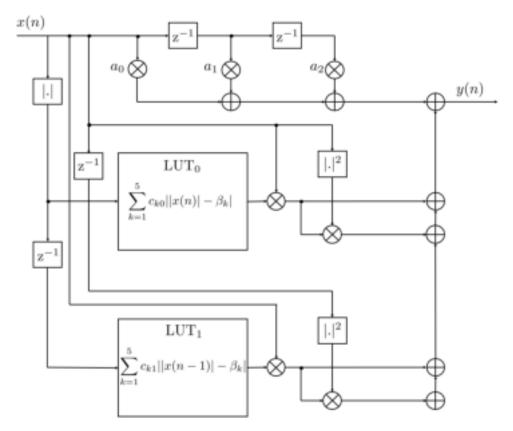
Figure 4.10: Implementation of optimal DVR model by LUT
