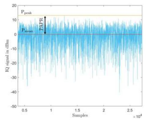
Figure 1.2: IQ data of LTE signal in dBm
