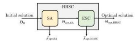
Figure 5.11: Block diagram of HHSC
