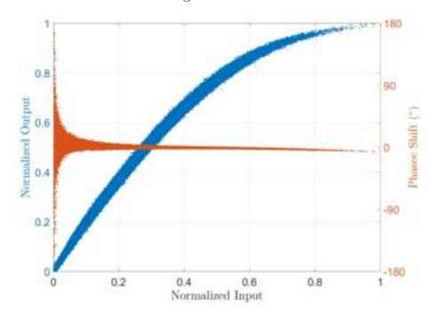
Figure 2.9: AM-AM & AM-PM curves of LDMOS PA for a 20 MHz LTE signal
