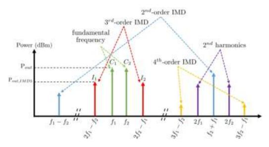
Figure 1.9: IMD products and harmonics of PA driven by two-tone signal
