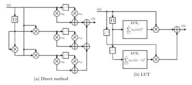
Figure 2.5: Implementation of an MP model with K=3 and M=1
