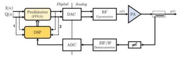
Figure 2.2: Baseband adaptive DPD with PA
