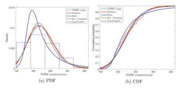
Figure 3.17: Fit probability distribution to data from experiment 1
