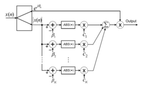
Figure 3.1: DVR basis function structure
