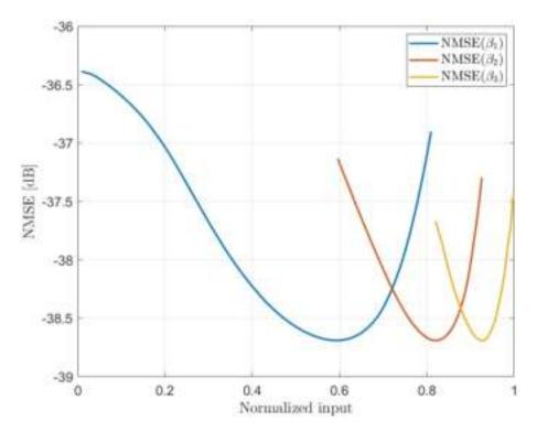
Figure 3.20: NMSE versus variation of  $\beta_i$  over  $I_i$  after random selection process where each NMSE( $\beta_i$ ) are unimodal
