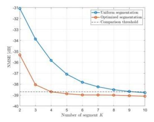
Figure 3.4: NMSE versus K with  $M_{lin}=2$  and M=1
