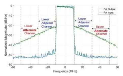
Figure 1.11: Upper and lower adjacent channels
