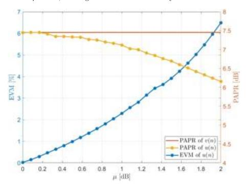
Figure 5.14: Behavior of EVM<sub>C</sub> and PAPR of v(n) versus  $\mu$
