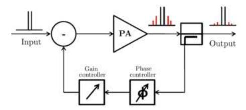
Figure 1.15: Principle of Feedback
