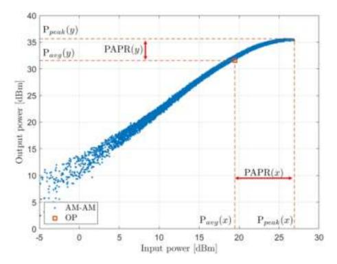
Figure 5.20: AM-AM characteristic using RF input-output signals
