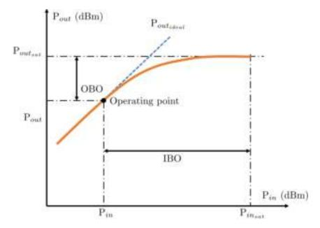
Figure 1.6: 1-dB compression point on AM-AM characteristic
