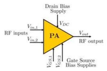
Figure 5.1: Block diagram of dual-input PA
