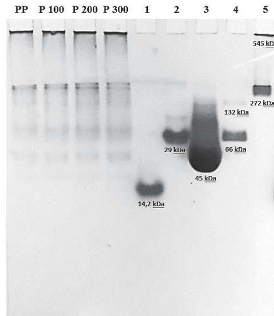
**Figure III.25.** Electrophoretic patterns of native 4–10% PAGE of native pea dispersion (PP) and PP dispersion treated by one single pass at a dynamic high pressure of 100 (P 100), 200 (P 200), 300 (P 300) MPa. Markers for native PAGE: alpha-lactalbumin (lane 1), carbonic anhydrase (lane 2), albumin chicken egg white (lane 3), bovine serum albumin (lane 4), urease from jack bean (lane 5).
