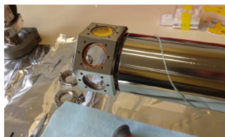
Figure 1 : Target windows holder of the IGLIAS set-up. The isotopic labeled gases are condensed at 8K on each window prior to irradiation. ZnSe IR-transparent windows (yellow window covered with a brown residue) are used, allowing IR spectroscopy monitoring during the irradiation.
