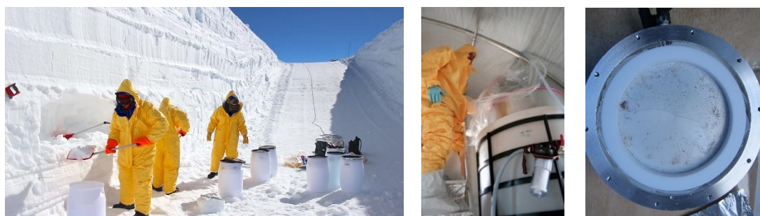
Figure 1-3: Blocks of snow are extracted from a trench with clean shovels and barrels (left). The extracted snow is subsequently melted in a clean closed-system (center). The melted snow is sieved by 30 µm mesh filters (right).
