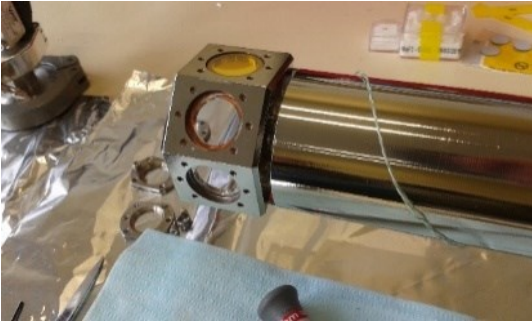
Figure 3-5: The IGLIAS window holder. Three 20 mm diameter windows can be mounted simultaneously in the holder (only one is present in the picture). Inside the IGLIAS chamber, the holder is cooled down to 9K by a cold finger.
