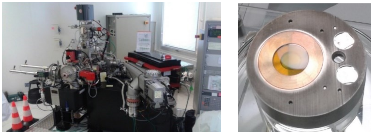
Figure 3-13: left, picture of the NanoSIMS at Institut Curie, Orsay, France. Right, ZnSe window in the NanoSIMS dedicated holder prior the analysis in June 2019. Half of the substrat window has been gold-coated.
