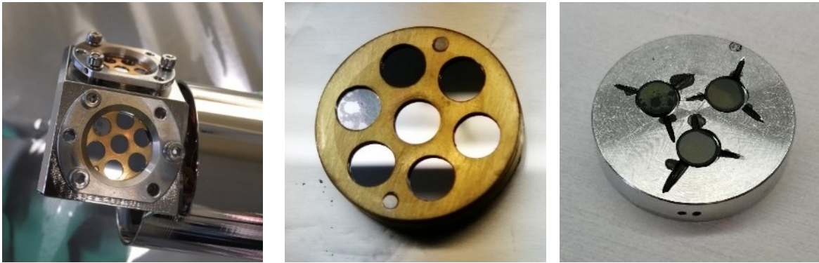
Figure 5-5. Left: visual aspect of the target Sd 4 at the end of the temperature ramp. Middle: close-up on the Sd4 window at the exit of the IGLIAS chamber. The 2020 experimental targets were made of seven 5mm large Si windows to insure a good charge evacuation during NanoSIMS analyses. The organic residue is visible on the leftmost window. Craters on the surface of the residue are certainly due to the formation of bubble during the temperature ramp. Right: dedicated aluminium holder for the NanoSIMS analyses. Three 2mm large Si windows from Sd4, Sd5 and Sd6 were fixed to the holder with a conductive carbon glue.
