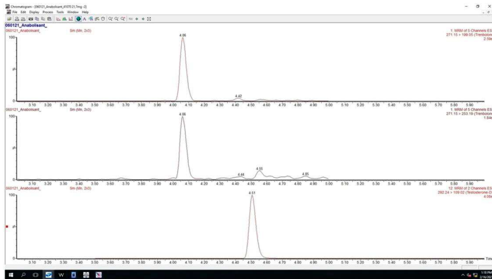
FIGURE 1 Chromatogram obtained after extraction of the arm hair specimen of subject n° 2. Trenbolone concentration was 15 pg/mg. From top to bottom: Two transitions for trenbolone and one transition for testosterone- d_3 (IS) [Colour figure can be viewed at wileyonlinelibrary.com ]
