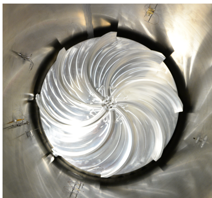
(a) Various sensors mounted on the periphery of the von Kármán cell
