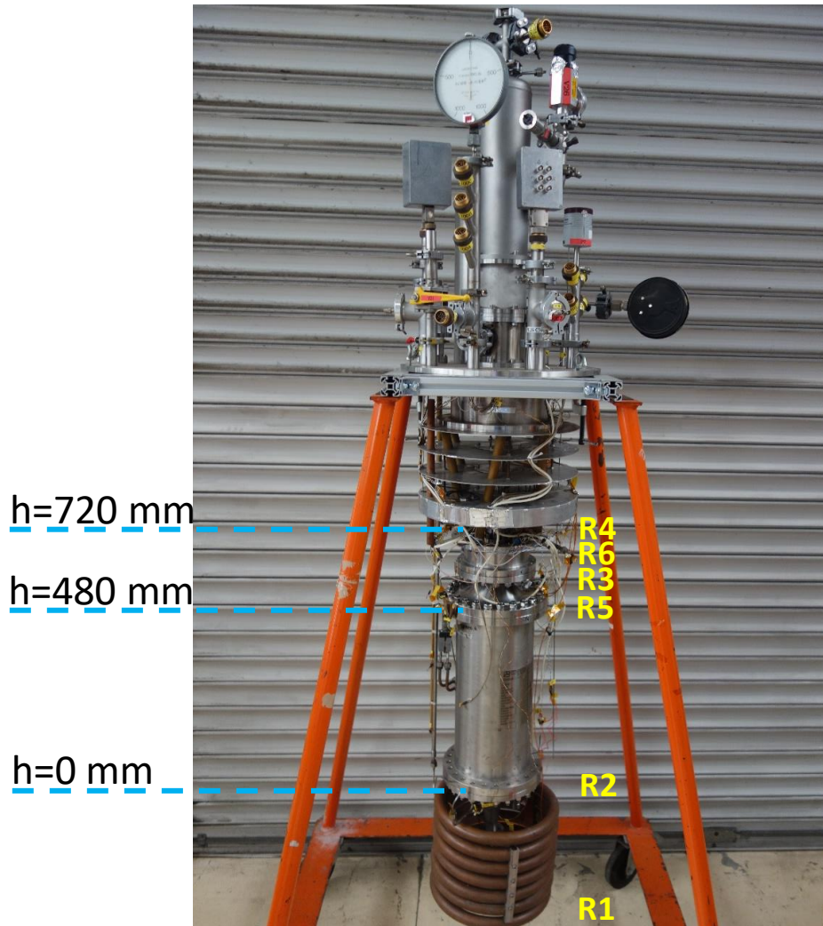
Figure IV.9: Actual view of the HEJET experimental facility [h denotes the level of helium in the saturated helium bath measured by the sensor of superconductor and R1 to R6 denotes the position (level) of 6 different resistances installed in the saturated helium bath]
