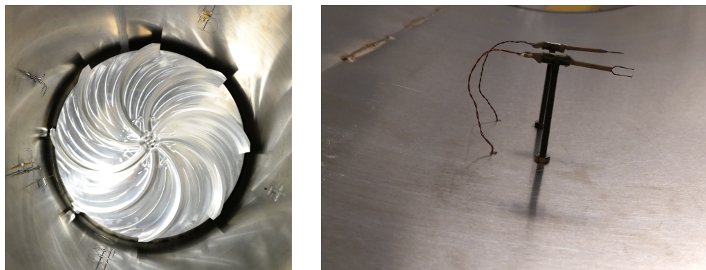
(a) Various sensors mounted on the periphery of the von Kármán cell (b) Hot-wire mounted at 40mm away from the wall of von Kármán cell
