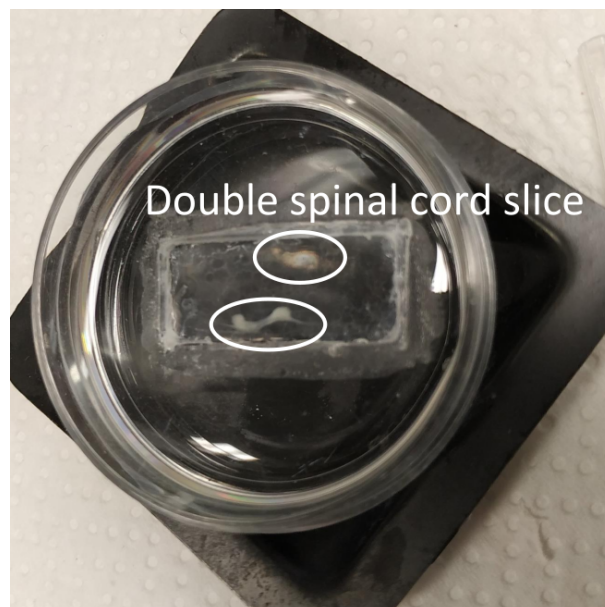
Figure 4.19: Double spinal cord slices incubated over a PDMS substrate and placed inside a Petri dish.
