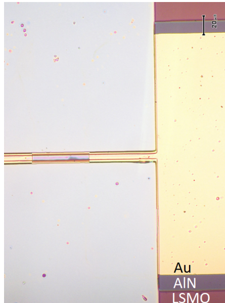
FIGURE 4.44: Clamped edge microscope image showing gold onto AlN onto LSMO perfectly aligned forming the full integrated actuation for the patterned bridges
