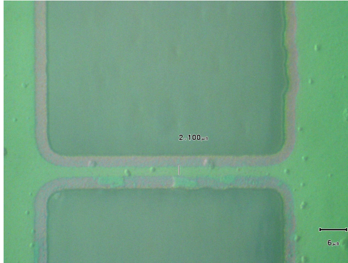
FIGURE 4.8: \text{SiO}_2 lateral etching evaluation after 30 minutes in HF bath at 20^\circ\text{C}
