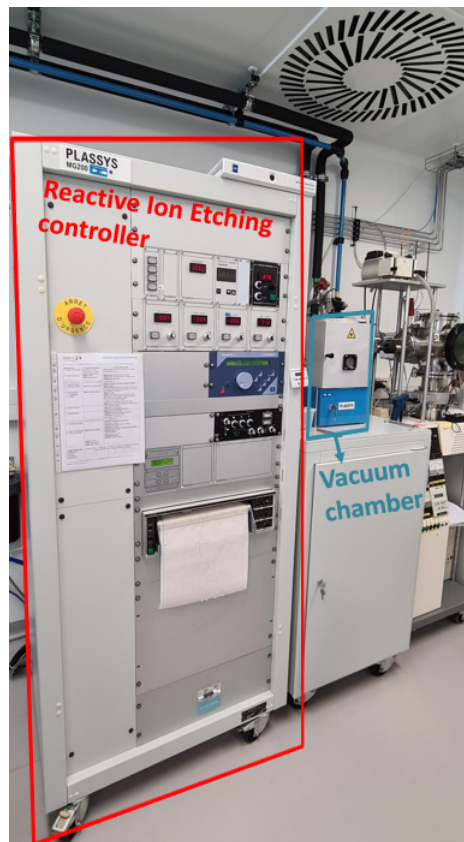
FIGURE 4.15: Reactive Ion Etching controller and its vacuum chamber (model PLASSYS MG 200) at the clean room at GREYC laboratory
