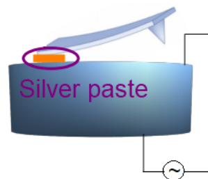
FIGURE 4.46: Setup for dynamic measurements on DHM using external piezoelectric disk
