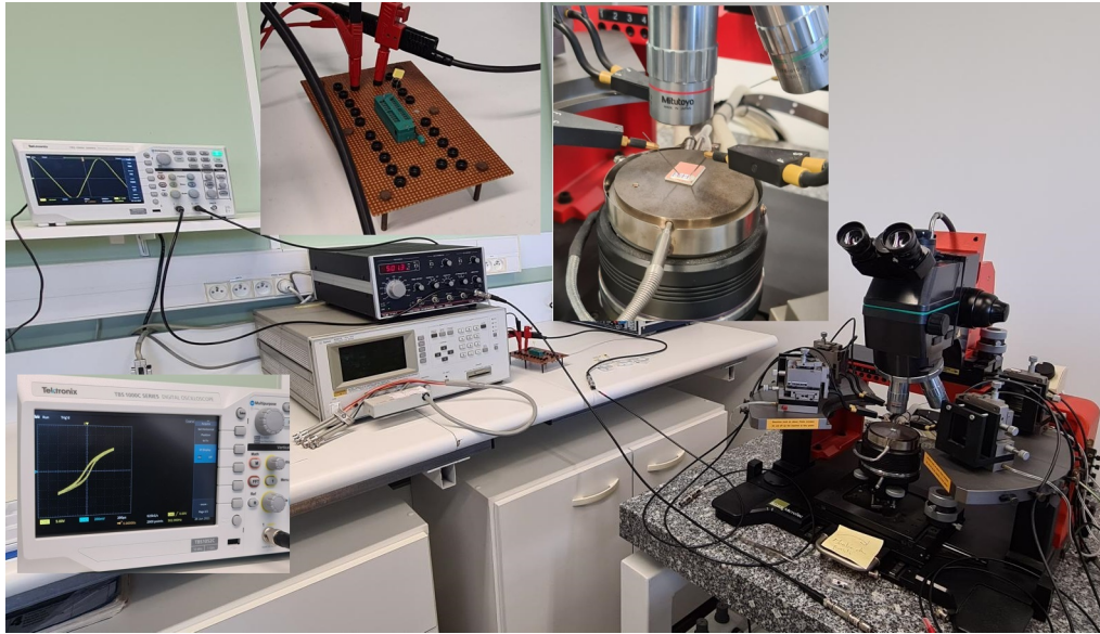
FIGURE 3.25: Measurement setup for P-E measurement at CRISMAT
