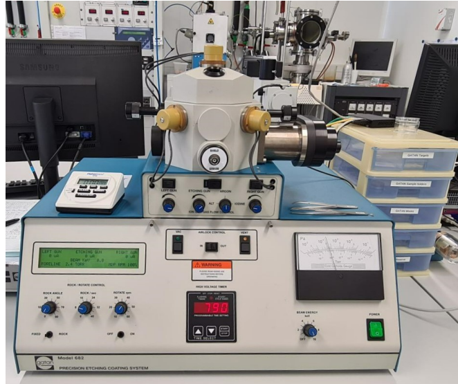
FIGURE 4.3: Front view of the precision etching and coating system used at the clean room at GREYC laboratory
