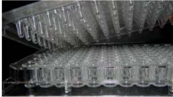
Figure 3 MBEC biofilm inoculator (adapted from Innovotech.ca)
