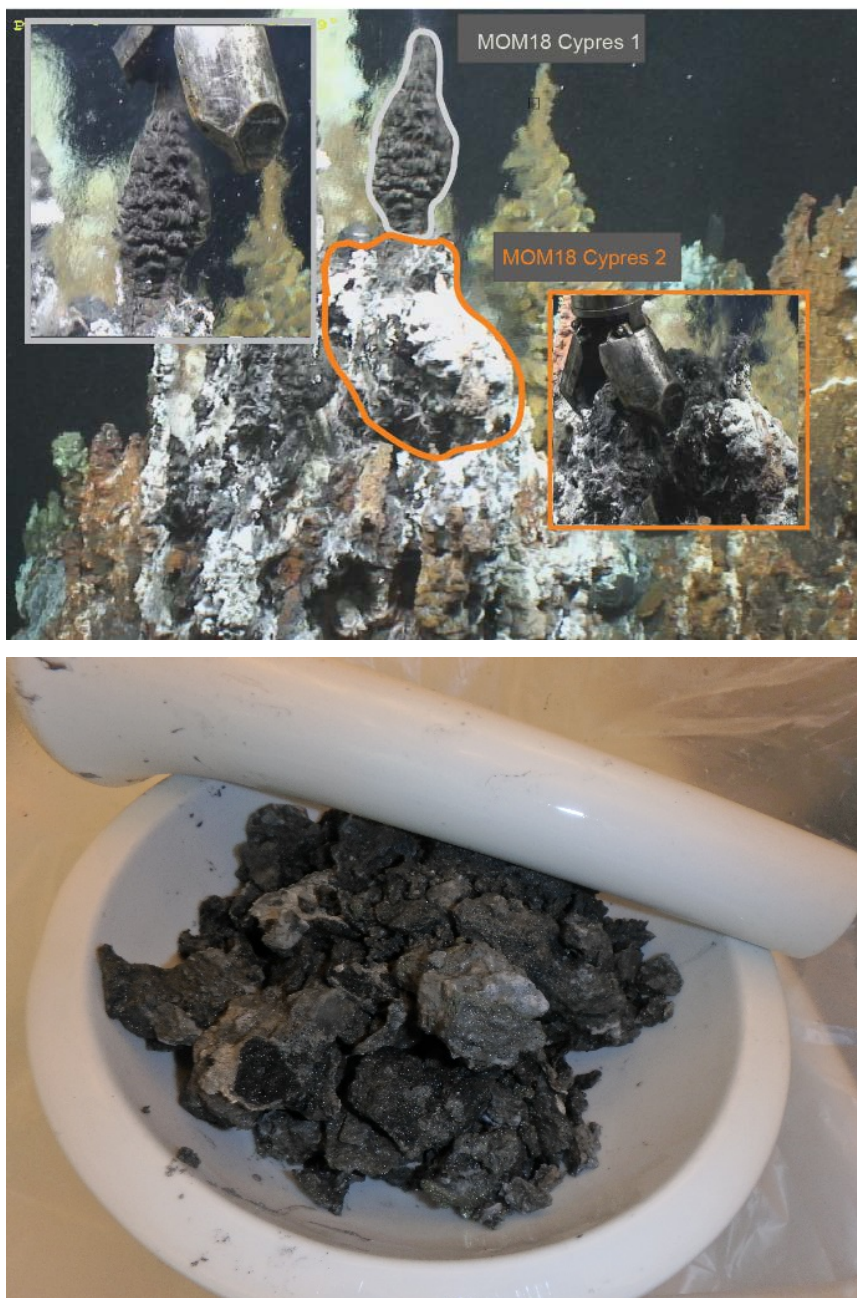
Figure 35 : Picture of hydrothermal chimney Cypres in 2018 detailing the upper and bottom parts (top). Picture of sample M18 Cyp 2 before crushing in a mortar (bottom).
