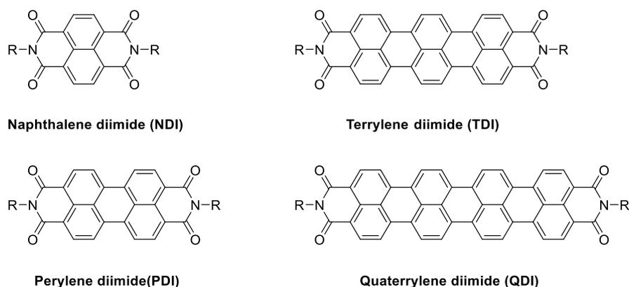
*Figure 17. Chemical structure of rylene diimide materials.*
