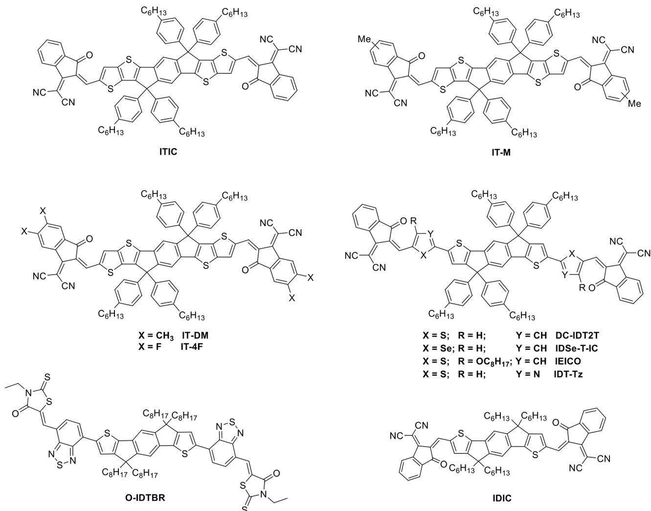
Figure 36. Examples of IDT and IDTT based NFAs.
