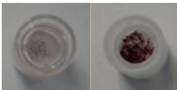
Figure 62. Normalized UV-visible of BTXI-CN and 11-NC-BTXI-CN evaporated thin films (30 nm) on quartz. Crucible images after total evaporation of the compounds BTXI-CN (left) and 11-NC-BTXI-CN (right).
