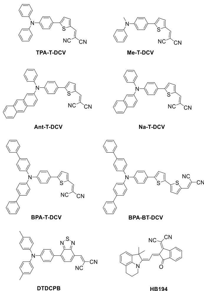
**Figure 13.** Chemical structures of push-pull small-molecule donors.
