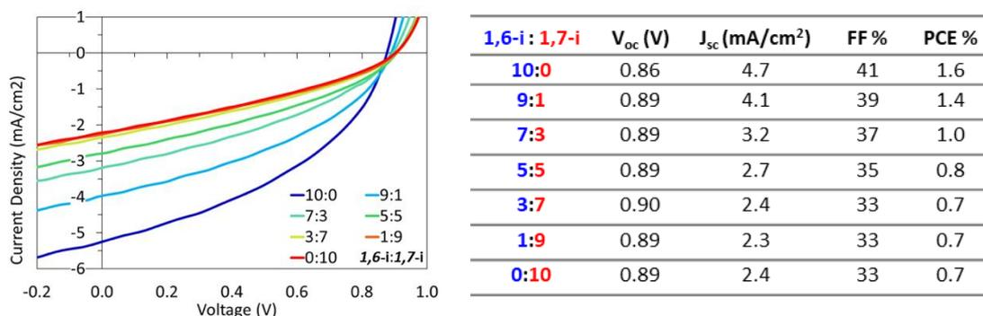
Figure 34 and Table 5.  $J$ - $V$  curves of devices (left) and organic solar cell device parameters (right) prepared with different ratios of 1,6-i and 1,7-i.
