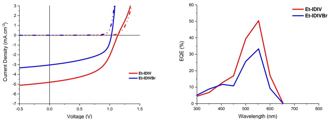
Figure 49. J-V and EQE curves obtained for ITO/NFA (10nm)/BF-DPB (10nm)/NHT169:NDP9 (45nm)/NDP9 (1nm)/Al (100nm) devices under illumination (solid line) and dark (dashed line). The J-V curves using **NHT169** are confidential, since this material is intellectual property of Heliatek.
