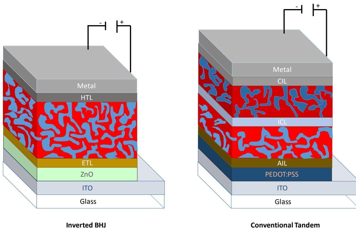
*Figure 8.* Architecture representation of inverted BHJ (left) and conventional tandem (right) devices. AIL stands for anode interface layer; ICL for interconnecting layer and CIL for cathode interface layer.
