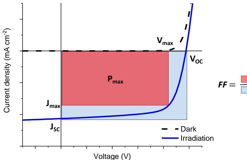
Figure 5.  $J$ - $V$  curves of an OSC in the dark and under illumination and extracted parameters.
