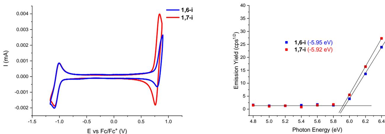
**Figure 29.** Cyclic voltammograms of **1,7-i** (red) and **1,6-i** (blue) at a concentration of 0.5 mM in 0.10 M  $Bu_4NPF_6/CH_2Cl_2$ ,  $100\text{ mV s}^{-1}$ , Pt working electrode (left). Photoelectron Spectroscopy in Air (PESA) and measured work function of **1,6-i** and **1,7-i** on spun-cast thin films (right).
