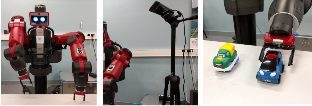
Figure 3.3: Experiment setup. Baxter robotics platform (left). Kinect sensor (middle). Subset of objects of interest (right).
