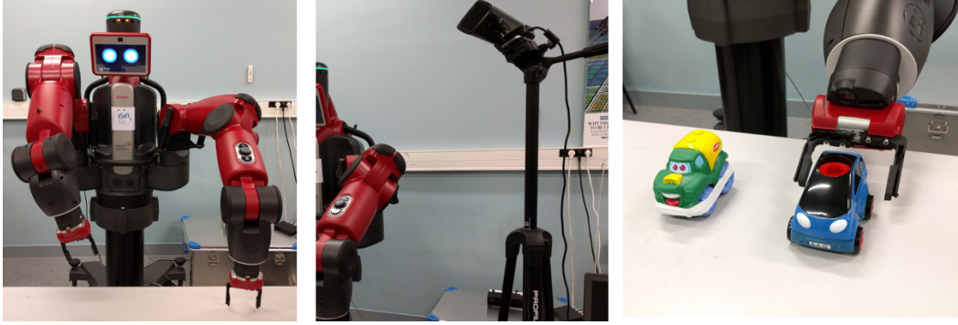
Figure 3.3: Experiment setup. Baxter robotics platform (left). Kinect sensor (middle). Subset of objects of interest (right).
