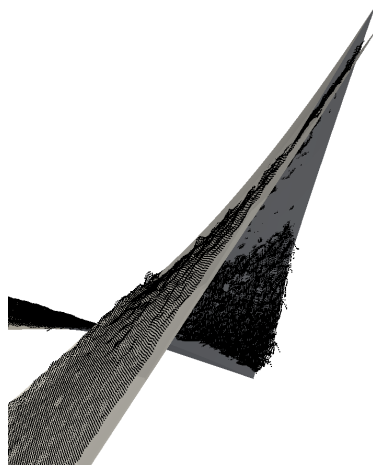
Figure 2.11: Unregularized FE shape measurement (black mesh) and different scales with different spline refinements with our CAD-based approach (gray surfaces) (def. scale fact. \times 30 ). This figure should be compared to Figure 1.5.
