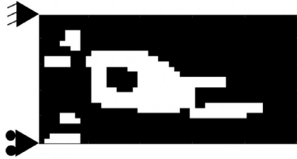
(c) Optimized geometry obtained for a volume fraction of 0.8, after filtering the raw optimal solution.
