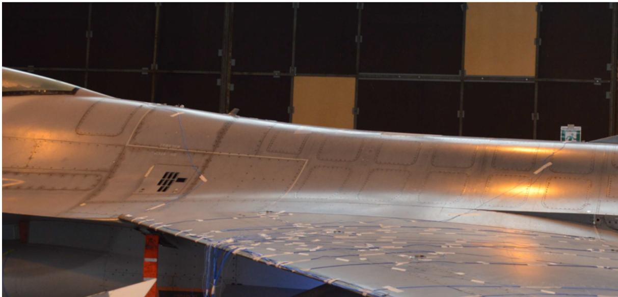
Figure 3: Dynamic strain sensors on the ground vibration testing of an F-16 aircraft, illustrating the coarse measurement point density on a large-scale test. Extracted from [[dos Santos et al. 2015](#)].
