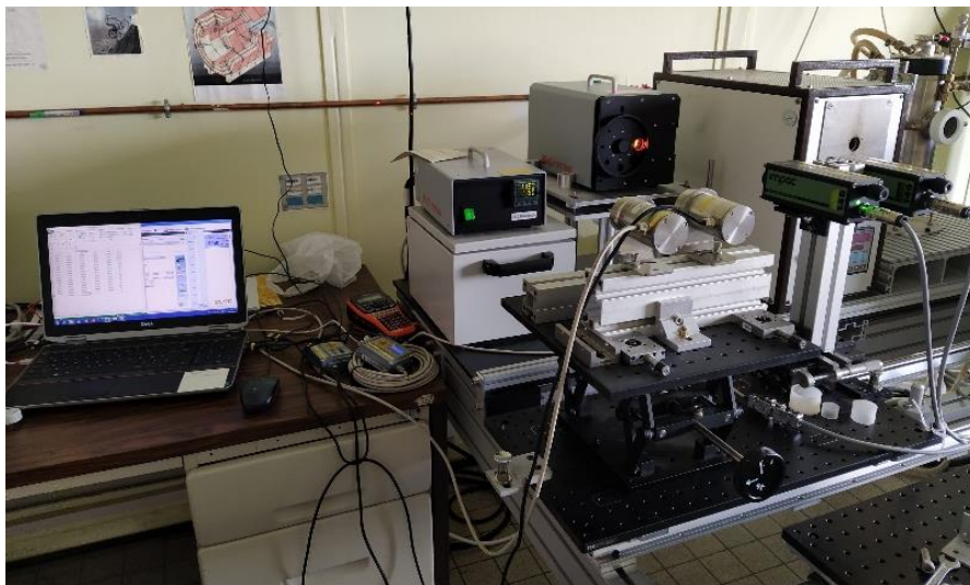
Figure 174. Pyrometer calibration set-up
