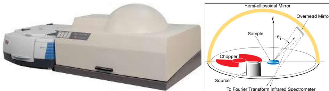
Figure 83. SOC-100 HDR with Nicolet 6700 FTIR spectrophotometer (left), principle of SOC-100 HDR (right)
