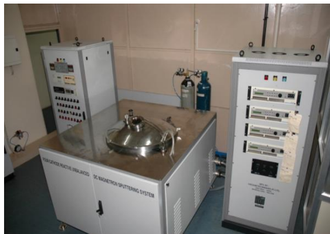
Figure 79. Four-cathode reactive unbalanced direct current magnetron sputtering system [311]
