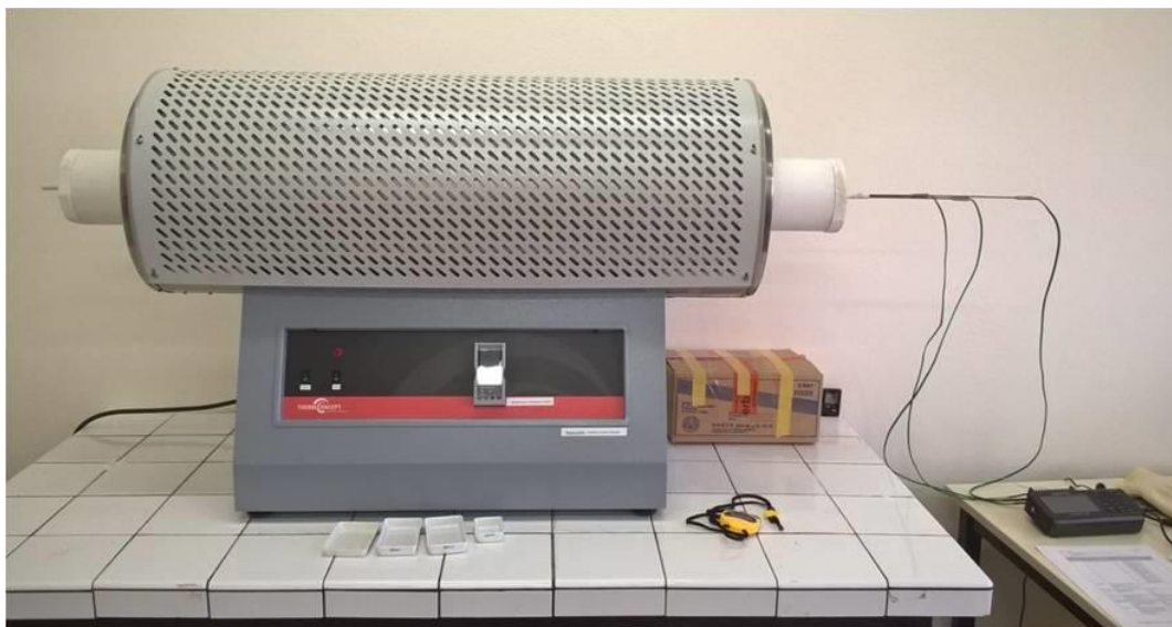
Figure 88. Thermconcept ROS 105/900/12 with Eurotherm 3508 temperature controller, insulating caps, independent thermocouples and Graphtec data logger
