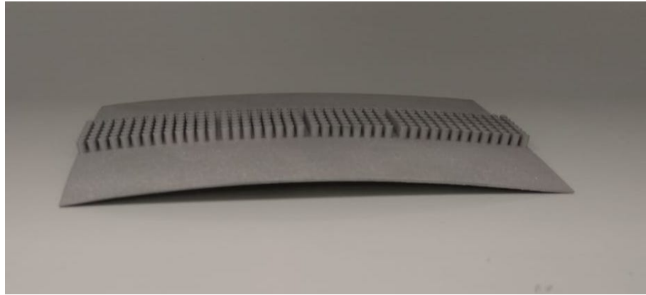
Figure 4.3: Warping issue due to thin plate that deformed because of residual stresses
