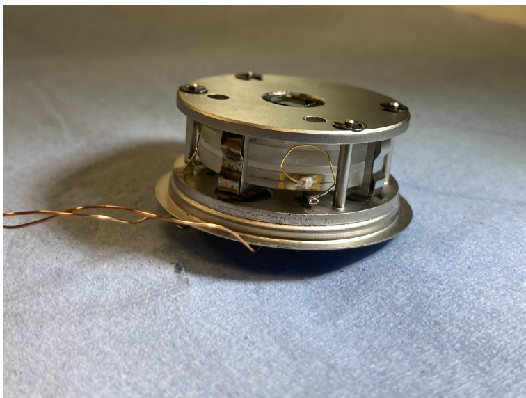
Figure B.3: Same as B.2 , with the BVA holder also in place. Note the hole on top of the structure, allowing the laser to pass by.
