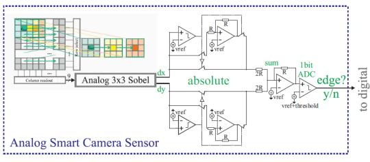
Figure 8 : circuit schematic for Sobel-like edge-magnitude-extraction (Soell et al. 2016)
