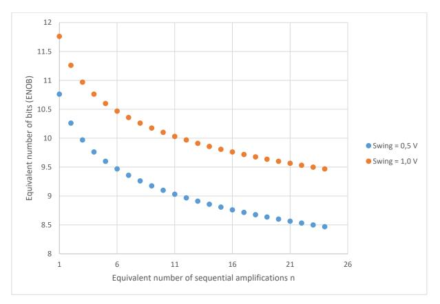
Figure 50 : Equivalent number of bits for two different pixel-intensity-voltage-swings V\_sig=V\_R, as a function of the equivalent number of sequential signal amplifications n. C\_H=100 fF,T=300 K.
