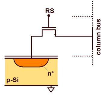
Figure 2 : illustration of the passive pixel in CMOS technology (Theuwissen 2007).
