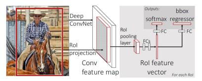
Figure 22 : diagram of the Fast R-CNN pipeline: "... An input image and multiple regions of interest (RoIs) are input into a fully convolutional networks. Each RoI is pooled into a fixed-size feature map..." (Girshick 2015)
