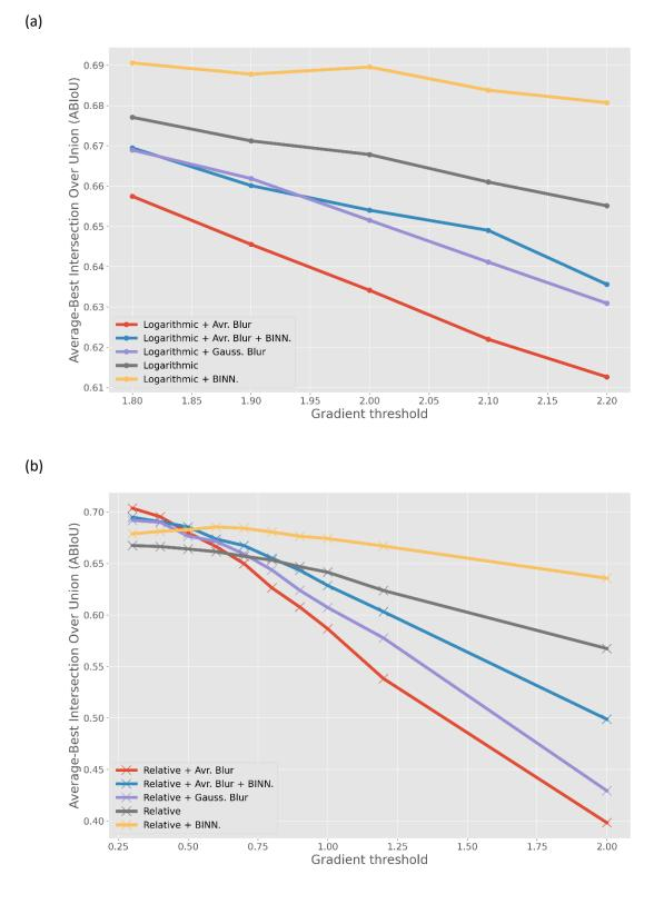
Figure 70 : Global ABIoU dependance upon the gradiend threshold for different architectures.
