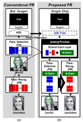
Figure 32 : "(a) Conventional face recognition system (b) Proposed face recognition system" (J.-H. Kim et al. 2019).
