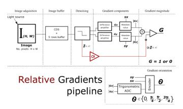
Figure 40 : adaptation from Figure 38 for relative gradients. The architecture segments added are colored in red.
