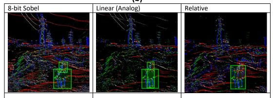
Figure 55 : example of an input image from PASCAL VOC2007 dataset (M. Everingham et al. n.d.; n.d.; Mark Everingham et al. 2015), and corresponding representations of the oriented edges map outputs from three different edge-extractors. The gray/red boxes represent the best ROI proposals after running Edge-Boxes on the edges-maps. Green means that the object was correctly including in the ROI, while red means that the object was not found (e.g. all ROIs where such that their IoU < 0.5).
