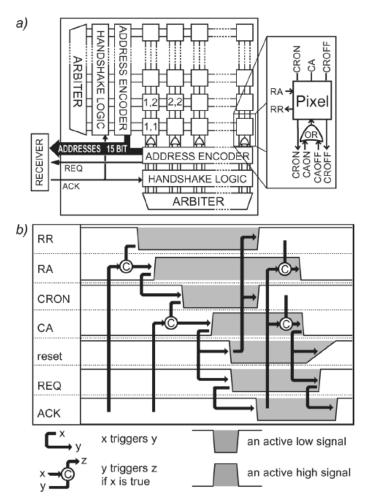
Figure 16 : example of the event-based read-out "(a) Block diagram. (b) Timing for a communication cycle for a single ON event..." (Lichtsteiner, Posch, and Delbruck 2008)
