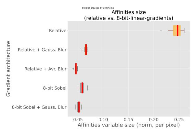
Figure 64 : affinities-variable-size comparison for architectures using relative linear gradients (8 ENOB).
