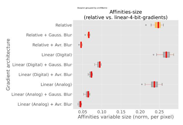
Figure 63 : affinities-variable-size comparison for architectures using relative and simple linear gradients (4 ENOB).
