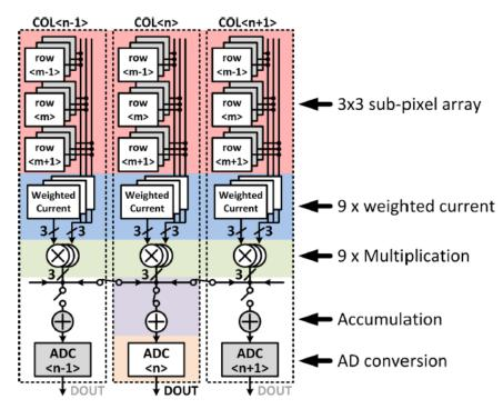
Figure 11 : diagram of the implemented pre-processing for MAC after PWD read-out (Hsu et al. 2021)
