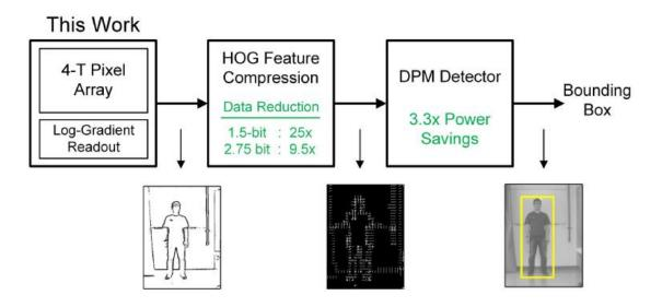
Figure 5 : logarithmic gradients object detection pipeline (Young et al. 2019).
