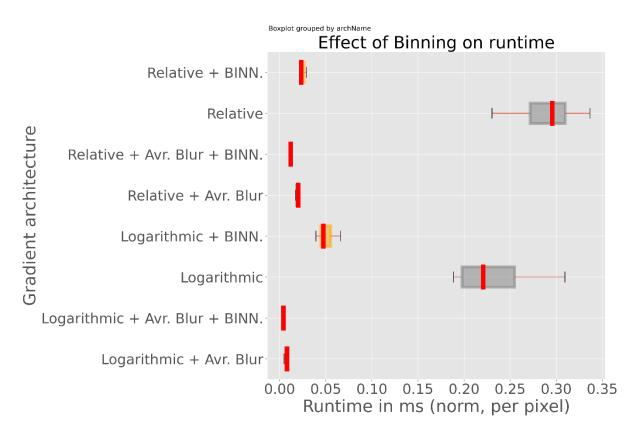
Figure 66 : normalized-runtime comparison for architectures using and not using 2x2 binning.
