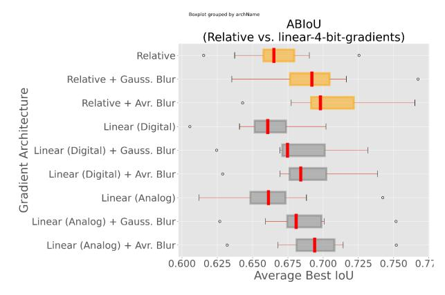
Figure 58 : global average best IoU comparison for architectures using relative and simple linear gradients (4 ENOB).
