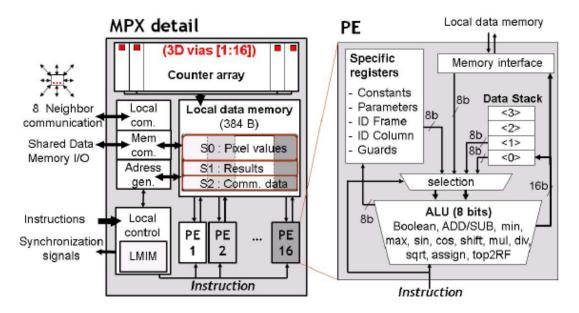
Figure 14 : diagram of the units implemented in the bottom layer (Millet et al. 2018)
