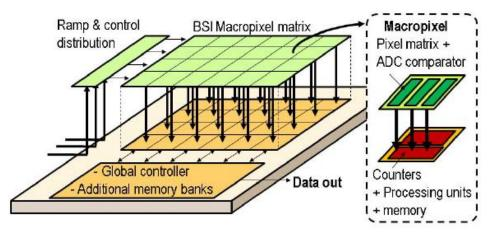
Figure 13 : illustration of the 3D-IC smart-image sensor (Millet et al. 2018)
