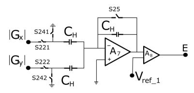
*Figure 47: circuit schematic for the summation and quantization stage.*
