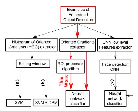
Figure 31 : Example of diagrams of pipelines for embedded integrated devices.
