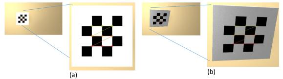
Figure 82 : result from OpenCV function for detecting the chessboard pattern corners at frame 10 (a) and at frame 20 (b).
