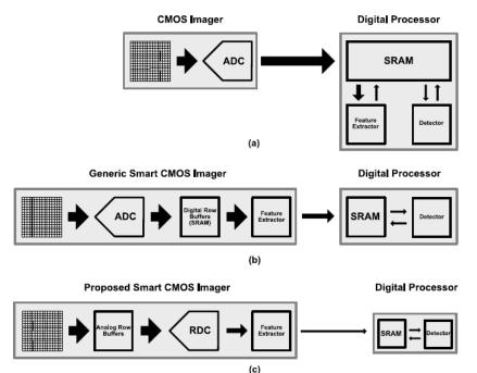
Figure 33 : (a) OD in general. (b) OD with embedded and digital pre-processing. (c) Their innovative approach with embedded digital and analog pre-processing. (Omid-Zohoor et al. 2018)
