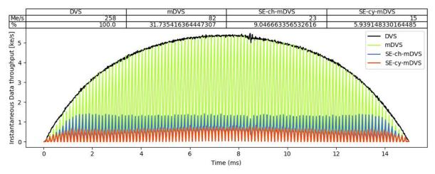
Figure 90 : instantaneous data throughput for the original DVS and for our three modifications. The table at the top presents the average data throughput.
