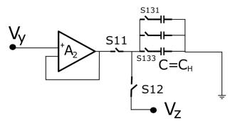
Figure 43: intermediary buffer schematic.
