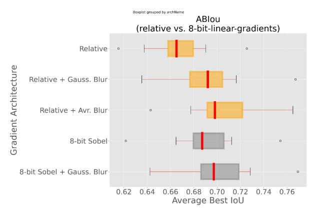
Figure 59 : global average best IoU comparison for architectures using relative and simple linear gradients (4 ENOB).
