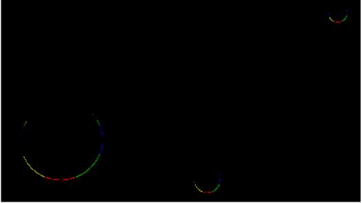
Figure 79 : example of a rendered frame from the output of the relative-edges extractor. Colors indicate the detected edge direction (blue: 90 deg, red: 0 deg, yellow: 45 deg, green: 135 deg).
