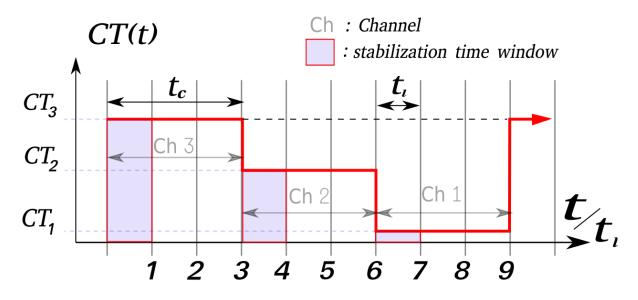
Figure 86 : our proposed modulation scheme (Cubero et al. 2020).
