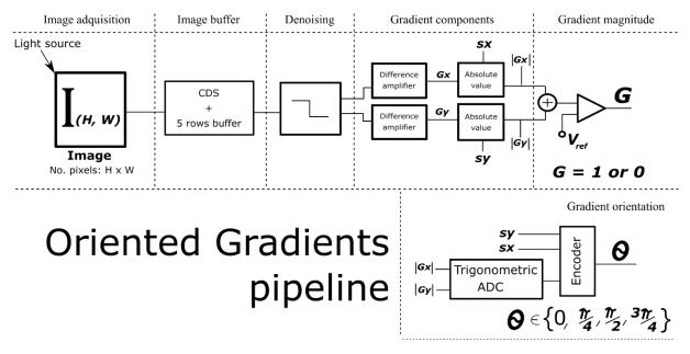
Figure 38: our proposed column parallel pre-processing pipeline for gradient computation.
