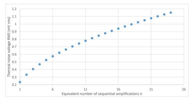
Figure 51 : RMS Thermal noise voltage ( $v(\sigma^2)$ ), as a function of the equivalent number of sequential signal amplifications n. C\_H=100 fF,T=300 K.
