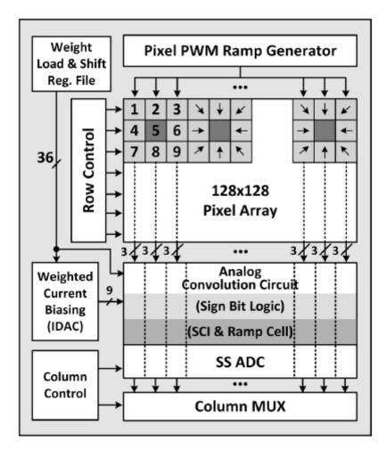
Figure 10 : system overview of the PWM pixels-matrix and programmable pre-processing (Hsu et al. 2021)
