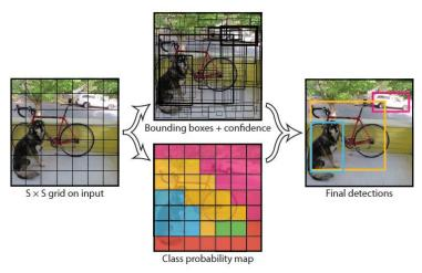
Figure 24 : illustration of the principle of the YOLO-pipeline: "...It divides the image into an S x S grid and for each grid cell predicts B bounding boxes, confidence for those boxes, and C class probabilities..." (Redmon et al. 2016).
