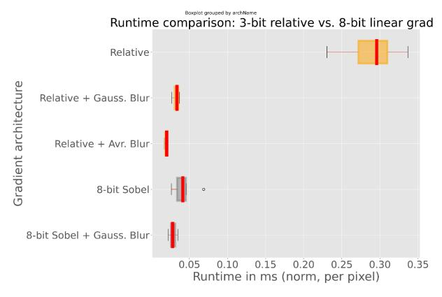
Figure 68 : normalized-runtime comparison for architectures using relative and 8-bit linear gradients.
