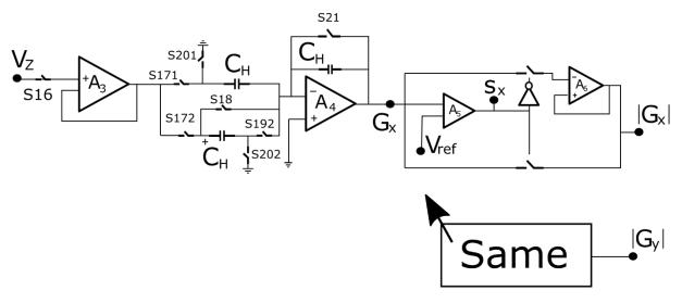
Figure 44 : schematic for computed gradient magnitude components.
