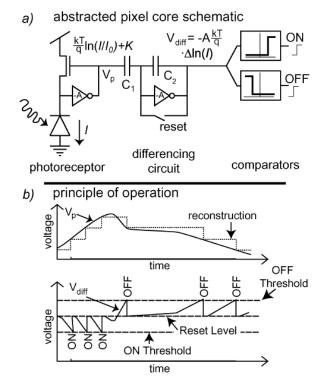
Figure 84 : "(a) Abstracted pixel schematic. (b) Principle of operation. In (a), the inverters are symbols for single-ended inverting amplifiers." (Lichtsteiner, Posch, and Delbruck 2008)
