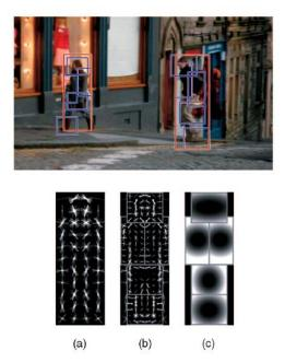
*Figure 21 : illustration of the principle of functioning of the DMP model. "(a) a coarse filter, (b) several higher resolution part filters, and (c) a spatial model for the location of each part relative to the root…" (P. F. Felzenszwalb et al. 2010)*
