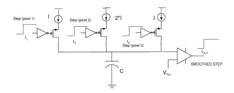
Figure 18 : example of a weighted average circuit in spike-domain (Ravinuthula and Harris 2004)
