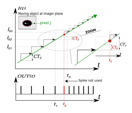
*Figure 87 : illustration of how an abrupt changing in CT triggers undesired spikes at the moment of the changing (Cubero et al. 2020).*
