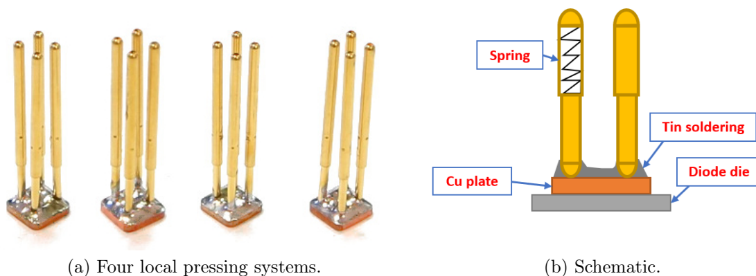
Figure 5.10: Local pressing system design.
