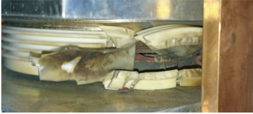
Figure 2.19: Diode exploded due to too high di/dt [128]
