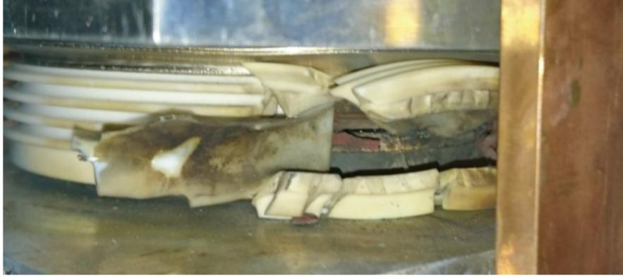
Figure 2.19: Diode exploded due to too high  $di/dt$  [128]
