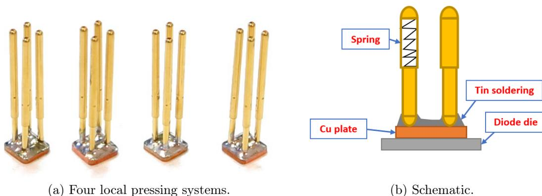
Figure 5.10: Local pressing system design.
