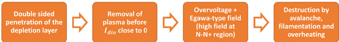
Figure 4.11: Chronology of the diode failure due to snap-off.
