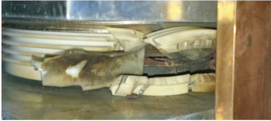
Figure 2.19: Diode exploded due to too high di/dt [128]
