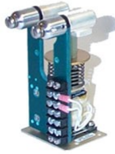
Figure 3.23: High-Voltage Relay used in the circuit. (Source: Ross Engineering)
