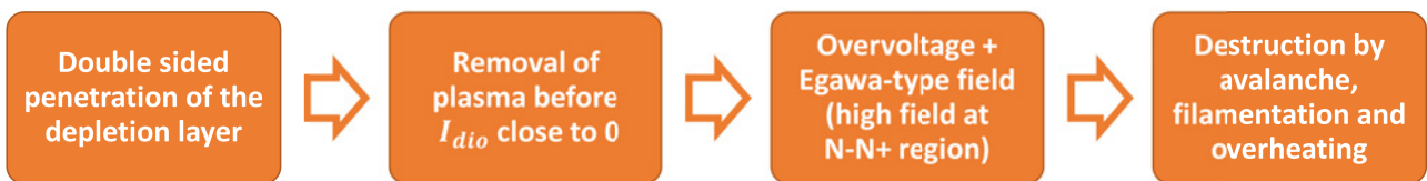
Figure 4.11: Chronology of the diode failure due to snap-off.
