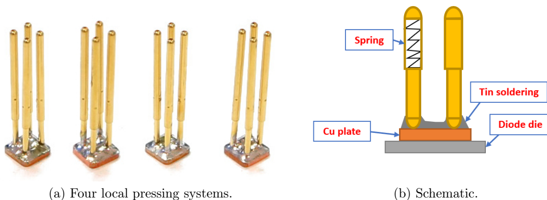
Figure 5.10: Local pressing system design.
