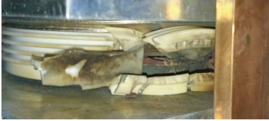
Figure 2.19: Diode exploded due to too high di/dt [128]
