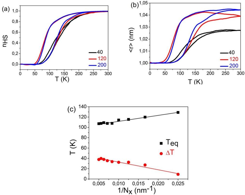
Figure 4. 4 Thermal dependence of the (a) HS fraction,  $n_{HS}$  and (b) average bond lengths
