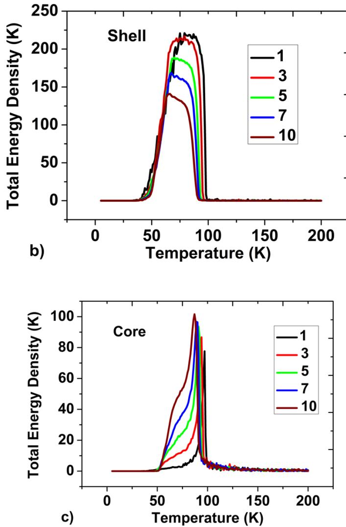
Figure 2. 18 Thermal variation of the total elastic energy density in the whole nanocomposite (a), (b) shell and (c) core, for different shell thicknesses, for the same core size,  $40 \times 40$ , along with the heating branch of the thermal hysteresis.
