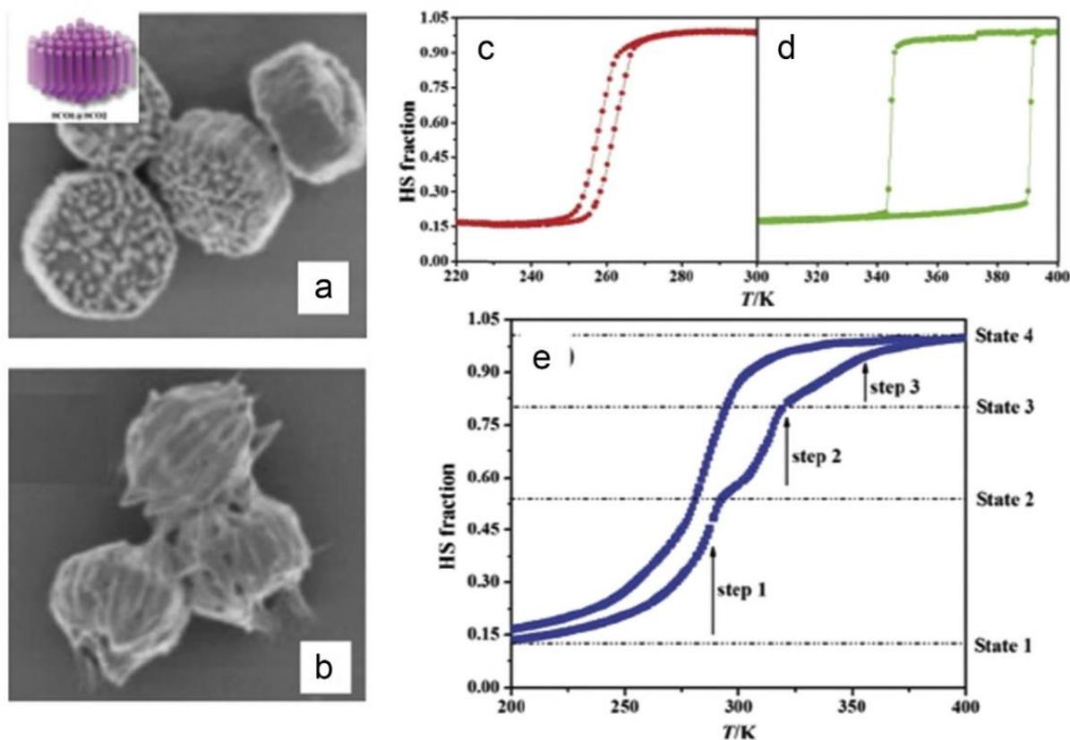
Figure 2. 3 SEM images of the SCO@SCO particles at an early stage (a) and final stage (b).  $cT \frac{1}{4} f(T)$  plots for the core alone (c), the shell alone (d), and the resulting core shells (e). Adapted from Ref.[52].
