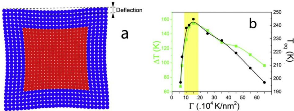
Figure 2. 8 (a) Example of a simulated squared core-shell nanoparticle using the electro-elastic model. The elastic misfit between the core and the shell induces a strain in the heterostructure, which the deflection calculation can quantify. (b) Effect of the shell stiffness on the thermoinduced spin transition of the core-shell nanoparticle: hysteresis width (green line) and equilibrium temperature (black line).
