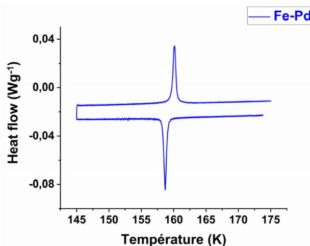
Figure 1. 22 DSC measurements showing the peaks of exo-, and endothermal transformations for the compound  $\{[Fe(2 - pytrz)_2[Pd(CN)_4]]\} \cdot 3H_2O$  [257].
