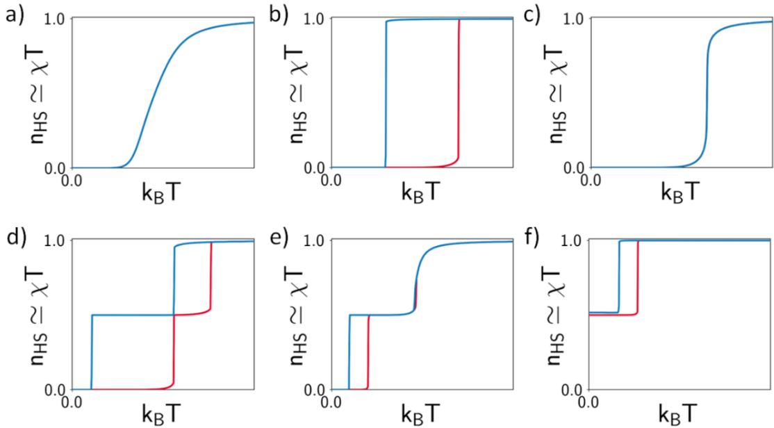
Figure 1.13 Heating (red) and cooling (blue) SCO curves (the fraction of high spins,  $n_{HS}$ , vs. temperature,  $T$ ) for (a) a crossover, (b) a one-step transition with hysteresis, (c) a continuous crossover, (d) a two-step transition with two first-order transitions, (e) a two-step transition with one first and one second-order transition and (f) an incomplete one-step transition with hysteresis [23].
