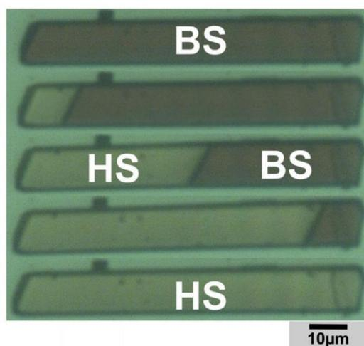
Figure 1. 24 Selection of images of a single crystal of the compound  $[Fe(NCSe)(py)_2]_2(m - bpyz)]$  placed under vacuum in a cryostat and illuminated by a light source of  $2.47mW$  during the heat-induced transition. The images are taken during the heating phase with a thermal scan of  $0.2 Kmin^{-1}$  [280]
