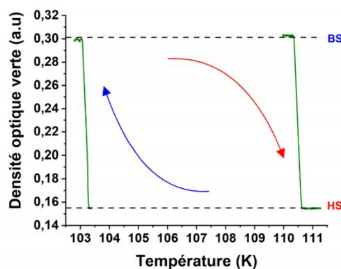
Figure 1. 25 Thermal evolution of the green optical density of a single crystal of the compound  $[Fe(NCSe)(py)_2]_2(m - bpypz)$  (Fig. 1.24), showing the hysteresis cycle of the spin transition.
