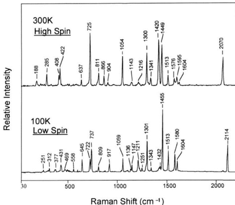
Figure 1. 7 Raman spectra of  $\text{Fe}(\text{phen})_2(\text{NCS})_2$  in the HS state (300 K) and LS state (100 K). In the range  $< 600 \text{ cm}^{-1}$  where the entropy values are maximized, the average of vibrational modes are  $\nu_{\text{av,HS}} = 298 \text{ cm}^{-1}$  and  $\nu_{\text{av,LS}} = 393 \text{ cm}^{-1}$  in the HS and LS states, respectively, leading to a ratio  $\nu_{\text{av,HS}}/\nu_{\text{av,LS}} \sim 1.3$ . [51]
