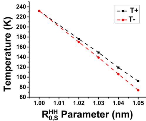
Figure 3. 6 High-spin shell lattice parameter dependence of the upper ( $T^+$ ) and lower ( $T^-$ ) transition temperatures of the core components, showing a clear vanishing of the thermal hysteresis for below the value,  $R_{0,S}^{HH} = 1.01$  nm, as a result of pressure effects exerted by the shell on the core due to the lattice parameter misfit.
