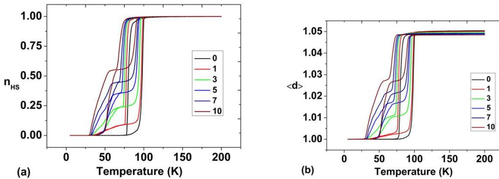
Figure 2. 12 Thermal variation of the total HS fraction (a) and the average lattice parameter (b) of the SCO nanocomposite for different shell thicknesses for a core size  $40 \times 40$ . The parameter values are:  $\Delta_S = 200 K$ ,  $T_{eq}^{shell} \approx 40 K$ ,  $\Delta_C = 450 K$ ,  $T_{eq}^{core} \approx 90 K$ . The used values of the elastic constants are:  $A_C = A_S = 10^5 K.nm^{-2}$  for nn interactions and  $B_C = B_S =$
