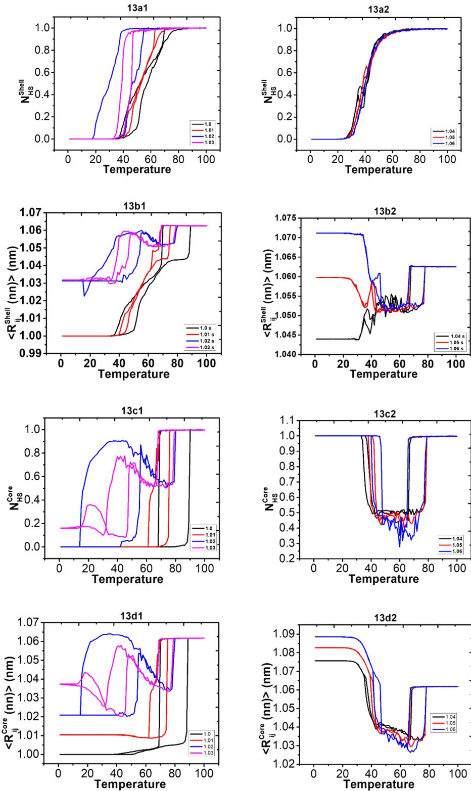
Figure 3. 13 Thermal variations of (a) the shell HS fraction and (b) average nn distance for different  $R_{0S}^{LL}$  values, varied from  $R_{0S}^{LL} = 1.0$  to  $1.06$  nm. (c) and (d) are the temperature dependences of the core HS fraction and average nn distance for the same  $R_{0S}^{HH}$  values. The
