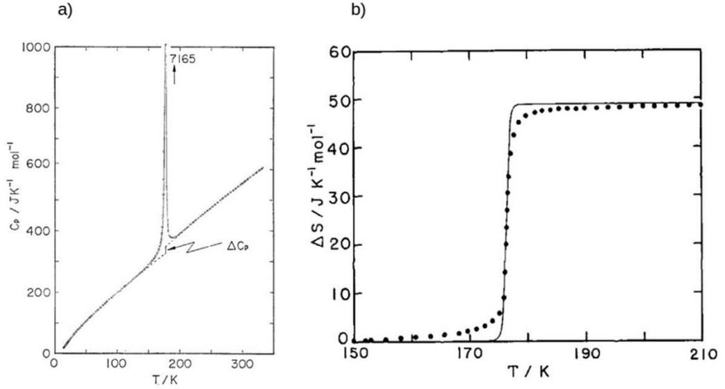
Figure 1.9 (a) Temperature dependence of the heat capacity of  $[Fe(phen)_2(NCS)_2]$  crystal.  $\Delta C_p$  corresponds to the discontinuity associated with the spin transition. (b) Temperature dependence of entropy variation of the same compound (full black circles). Straight line corresponds to a fit using the so-called domain model [59].
