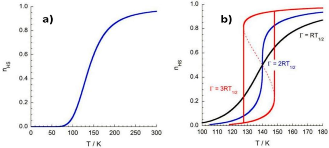
Figure 1.15 (a) Fraction of HS-state molecules  $n_{HS}$  as function of temperature, ( $\Delta H = 7\text{kJ}\cdot\text{mol}^{-1}$ , and  $\Delta S = 50\text{J}\cdot\text{K}^{-1}\cdot\text{mol}^{-1}$ ). (b) Fraction of HS-state molecules  $n_{HS}$  as function of temperature, ( $\Delta H = 7\text{kJ}\cdot\text{mol}^{-1}$  and  $\Delta S = 50\text{J}\cdot\text{K}^{-1}\cdot\text{mol}^{-1}$ ) [46].
