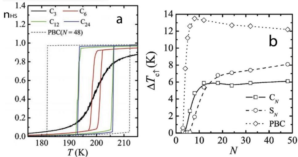
Figure 2. 4 (a) The fraction of the unit in the HS state in an equilibrium state,  $n_H$ , for various sizes of cubic particles. For comparison, the result at  $N \approx 48$  with the PBC is also shown. (b) Size dependence of the width of the thermal hysteresis  $\Delta T_c$  for cubic particles ( $C_N$ ), spherical ones ( $S_N$ ) and the PBC case.
