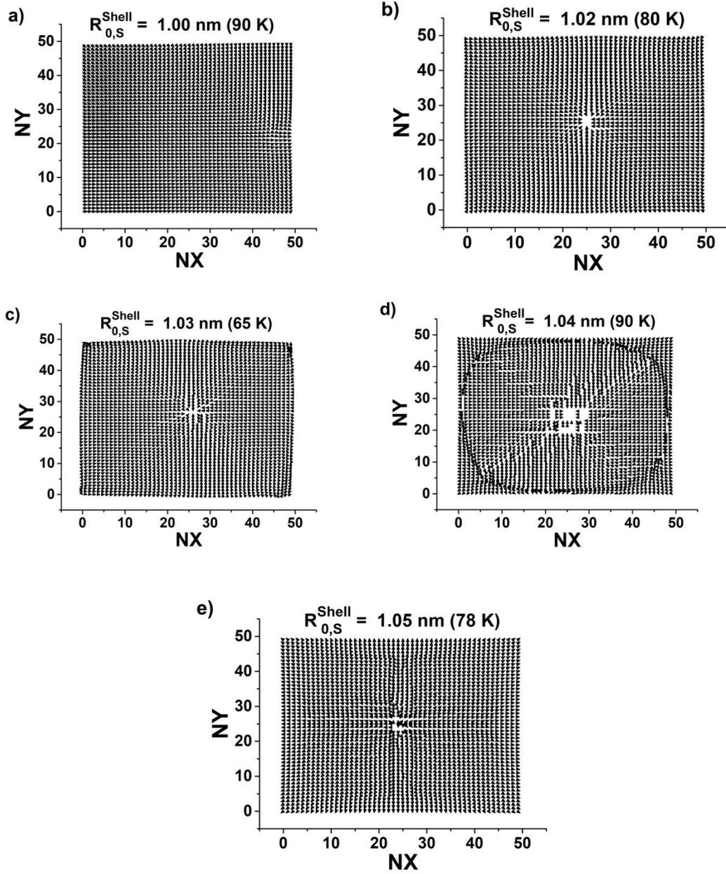
Figure 3. 10: Displacement fields for the different HS shell lattice parameter values a)  $R_{0,S}^{HH} = 1.00$  nm b)  $R_{0,S}^{HH} = 1.02$  nm c)  $R_{0,S}^{HH} = 1.03$  nm d)  $R_{0,S}^{HH} = 1.04$  nm and e)  $R_{0,S}^{HH} = 1.05$  nm, corresponding to the situations depicted in Figs. 3.9a-e. The LS state, common to all figures, was used as a reference state for the calculations of the displacement field (see Eq. (3.10)).
