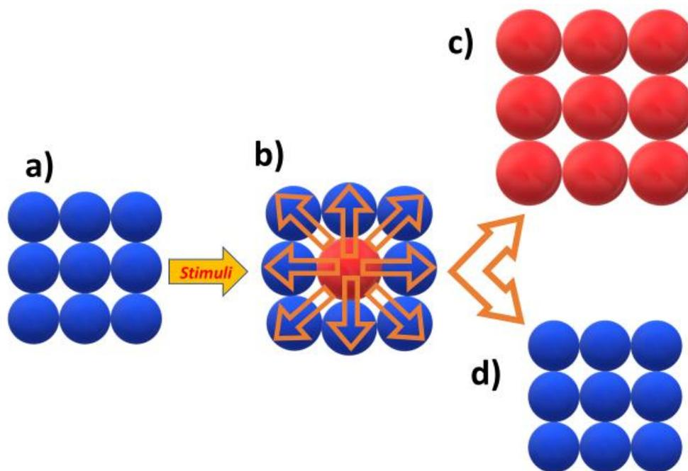
Figure 1.11 Simplified representation of collective mechanisms in the case of a highly cooperative SCO compound a) Molecules in the LS state. b) The central molecule transits towards the HS state, which implies a lattice deformation, and the molecule wants to expand (arrows). As a result, c) either the neighbors transit towards the HS state or d) the molecule returns to the LS state
