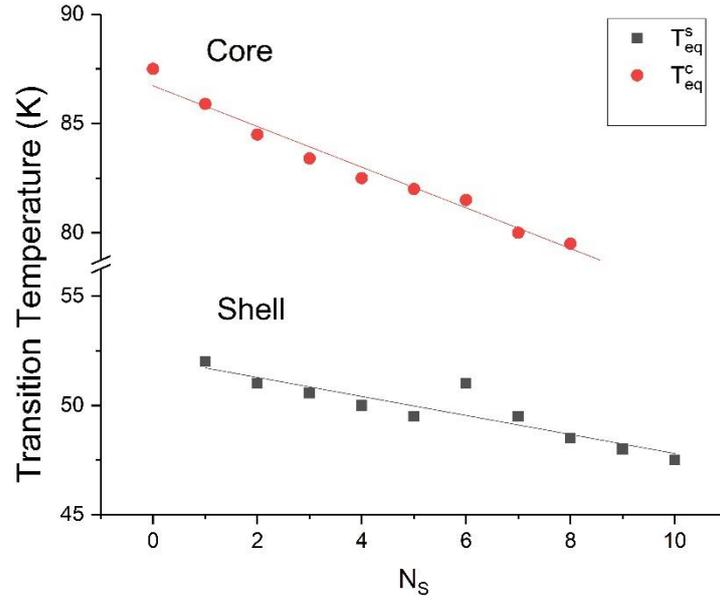
Figure 2.13 Average equilibrium transition temperatures of the shell and the core components of the nanocomposite deduced from MC simulations of Fig. 2.12. Bold lines are the best linear fitting.
