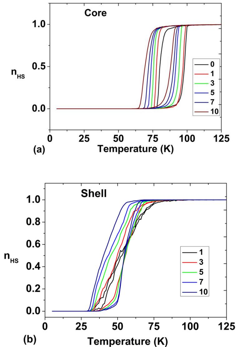
Figure 2. 14: Thermal response of the HS fraction of the core (a) and shell (b) of the SCO nanocomposite, for different shell thicknesses (from  $N_s = 0$  to 10), corresponding to the results of Fig. 2.12.
