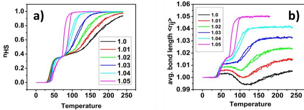
Figure 5. 2 Showing total  $n_{HS}$  fraction, and  $\langle r_{i,j} \rangle$  avg. bond lengths for core-shell architecture for a predefined interface with misfit in HS state of SCO, which qualitatively is similar to what we observed and discussed in chapter 3, with some differences such as hysteresis width, transition temperature, etc.
