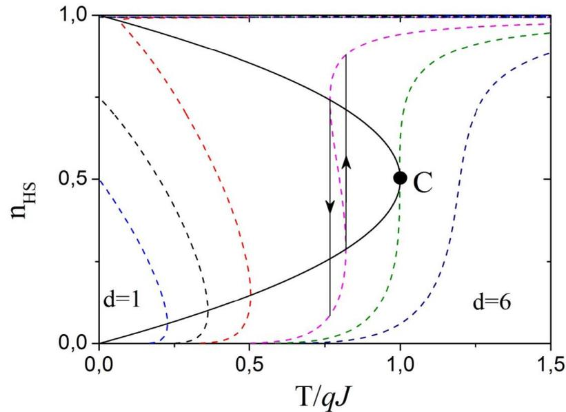
Figure 1.14 Thermal behavior in reduced coordinates calculated from equation (1.25) for  $g = 150$  and the values of  $d = \Delta_0/qJ = 1, 2, 3, 4, 5$  and  $6$  in the mean field approximation. The point C obtained for  $d_c = \Delta_0/qJ = \ln g \sim 5.01$  is the critical point. Hence for  $d < d_c$  there is no longer any first order transition. The solid line is the spinodal curve. Adapted from reference [154]
