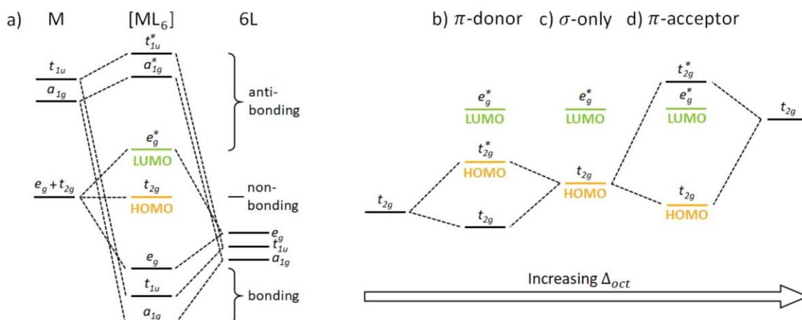
Figure 1. 3 Molecular orbital energy level diagrams for ML<sub>6</sub>, showing (a) the influence of  $\sigma$ -bonding and (b-d)  $\pi$ -bonding on the molecular orbitals. The energy difference between the highest occupied molecular orbital (HOMO) and lowest unoccupied molecular orbital (LUMO) strongly depends on the type and strength of the  $\pi$ -bonding, decreasing for stronger (b)  $\pi$ -donation and increasing for stronger (d)  $\pi$ -acceptance. Adapted from [23]
