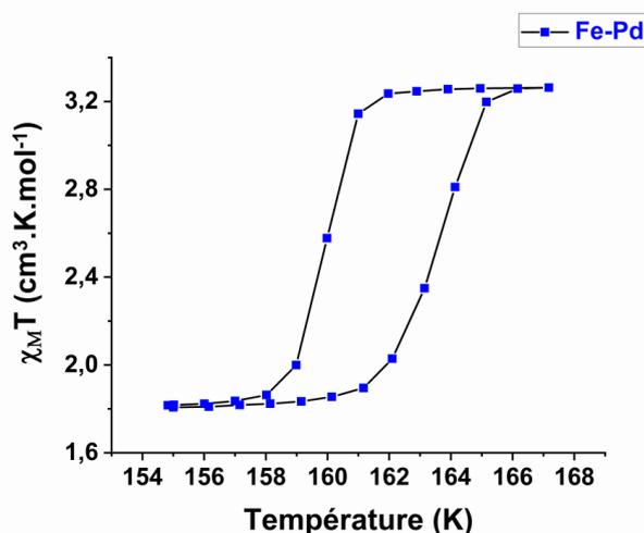
Figure 1. 21 Thermal evolution of the product  $\chi_m \cdot T$  for the compound  $\{[Fe(2 - pytrz)_2[Pd(CN)_4]] \cdot 3H_2O\}$  [257].
