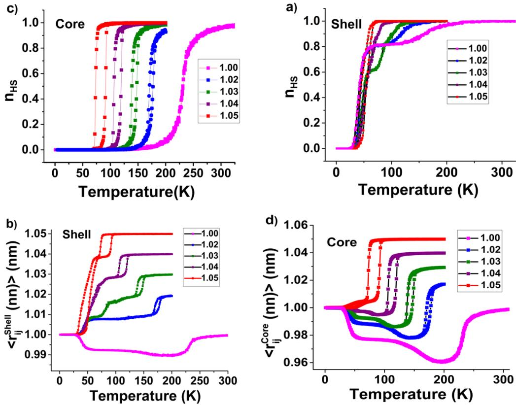
Figure 3. 4 Thermal variations of (a) the shell HS fraction and (b) average nn distance for different  $R_{0,S}^{HH}$  values, varied from  $R_{0,S}^{HH} = 1.0$  to 1.05 nm. (c) and (d) are the temperature dependences of the core HS fraction and average nn distance for the same  $R_{0,S}^{HH}$  values. The other lattice parameter values are given in Table I. The other model parameters are given in the text.
