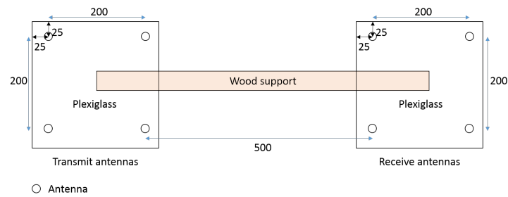
Figure 5.31: Antennas position on the support
