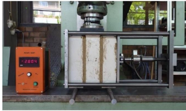
Figure 1.17. Triplet test specimens and setup (from [261])
