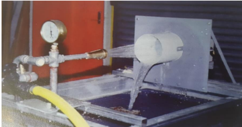
Figure 1.15. Setup of the spray erosion test (from the Australian earth building handbook (HB 195))
