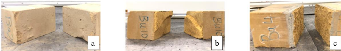
Figure 5.11. Examples of the three observed failure modes, A1 (a), A2 (b) and C (c)
