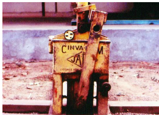
Figure 1.1. Cinva Ram, the first press for compressed earth blocks
