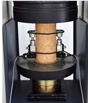
Figure 1.10. Example of direct compression test on cylindrical sample (from [189])
