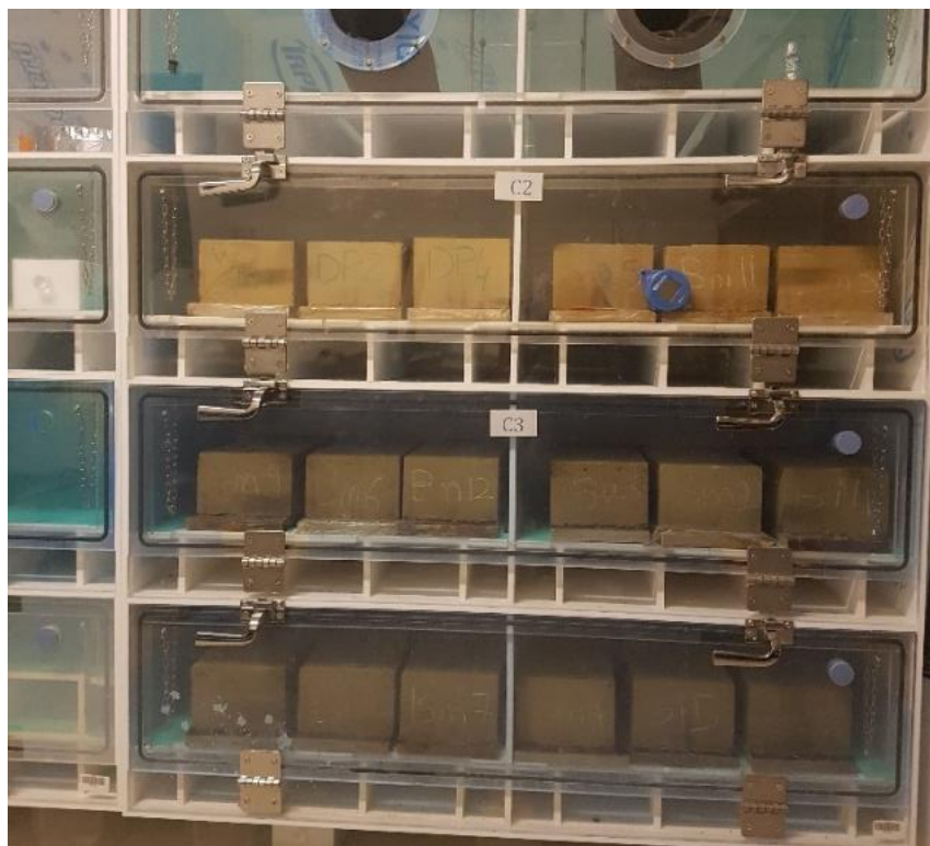
Figure 5.1. Blocks stored in controlled conditions of temperature and relative humidity
