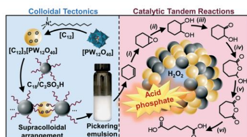
Fig. 1 Colloidal Tectonics concept based on [C_{12}]_3[PW_{12}O_{40}] ( C_{12} -POM) and C_{18}/C_3SO_3H NPs applied to the synthesis of dicarboxylic acids (e.g., adipic acid) starting from cyclic alkenes (e.g., cyclohexene).
