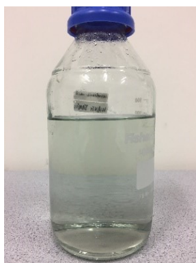
Figure 3.4. Green solution after experiments due to the existence of ion \text{Fe}^{2+} .
