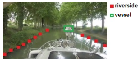
(b) Multiple rectangular bounding boxes are drawn to delimit objects with corresponding class labels.
