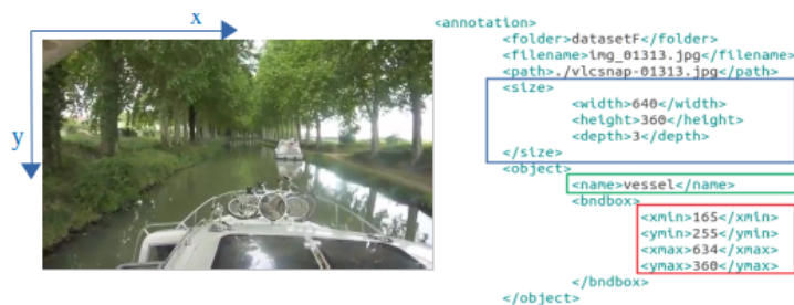
(a) The details of a labeled object (ship): The blue, green and red rectangles indicate the shape of the image in the left, the object name, and its location, respectively.
