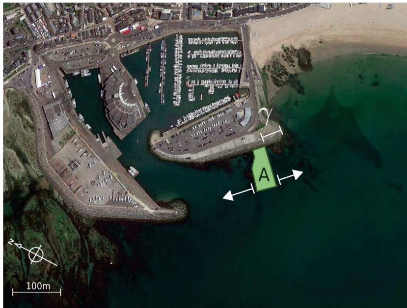
Figure 1.15: Parameter \gamma defining the groyne
