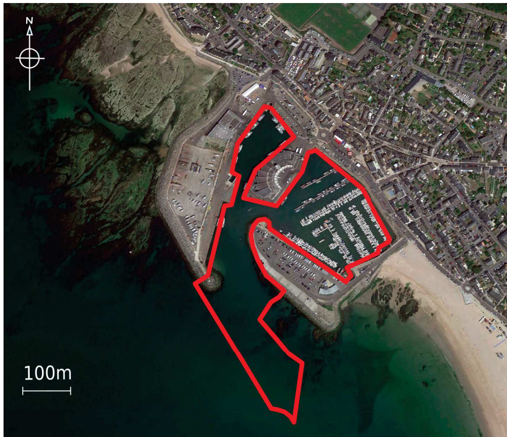
Figure 1.9: The inner border (red) of the optimal configuration of the port, resulting from the minimization of energy. We observe an extended jetty and a wide mole.
