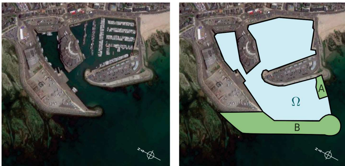
Figure 1.3: Illustration of La Turballe port. Left : The port in its initial state. Right : The port with the two additional structures considered in this study: mole A and jetty B.
