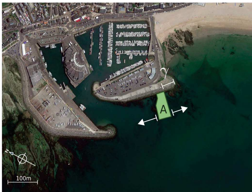
Figure 1.15: Parameter \gamma defining the groyne
