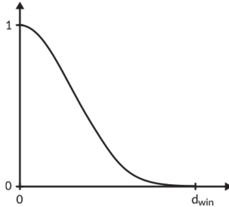
Figure 4.8: Weighting function w , equal to 1 closest to the present wave and decreases exponentially as the distance seaward increases
