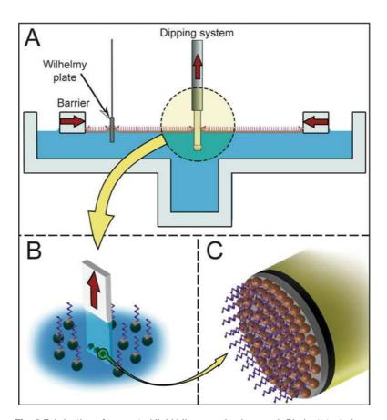
**Fig. 2** Fabrication of supported lipid bilayers using Langmuir Blodgett technique. (a) Schematic view of the Langmuir balance; (b) zoom on the dipping system made in polyether ether ketone (PEEK), chemically modified and biologically inert. Glass rods with mica disk glued at the top, similar to those shown in Fig. 1, are inserted in holes in the polymer plate; (c) zoom on mica, glued at the top of a glass rod and covered by a lipid monolayer
