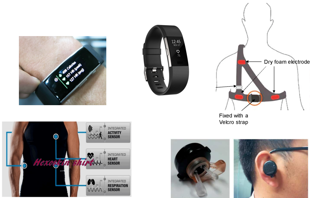
FIGURE 1.5: Some wearable devices that monitor physiological signals
